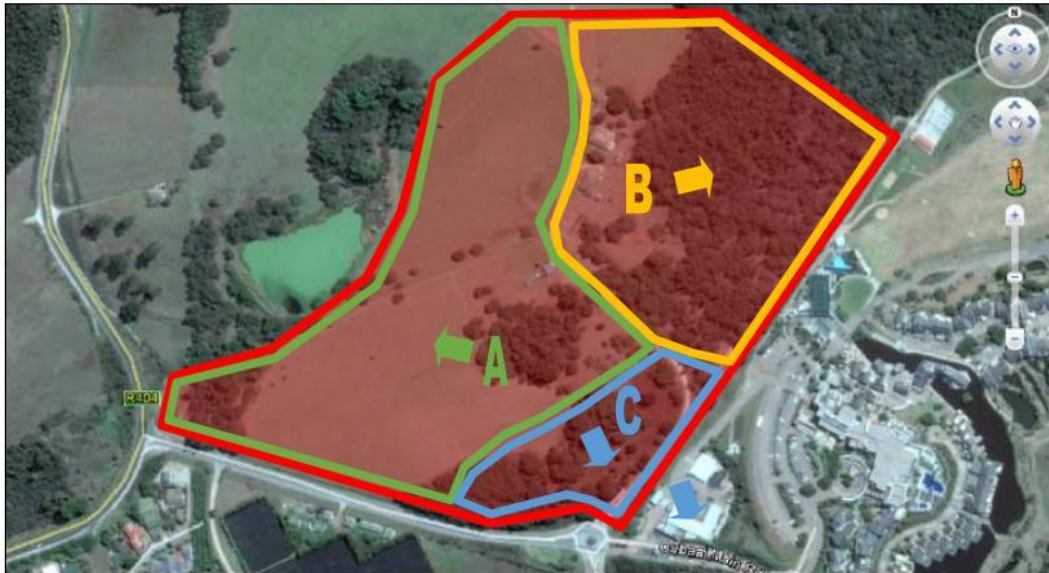
Figure 6: Sewer Drainage Zones (Source: Element Consulting Engineers, 2019)
