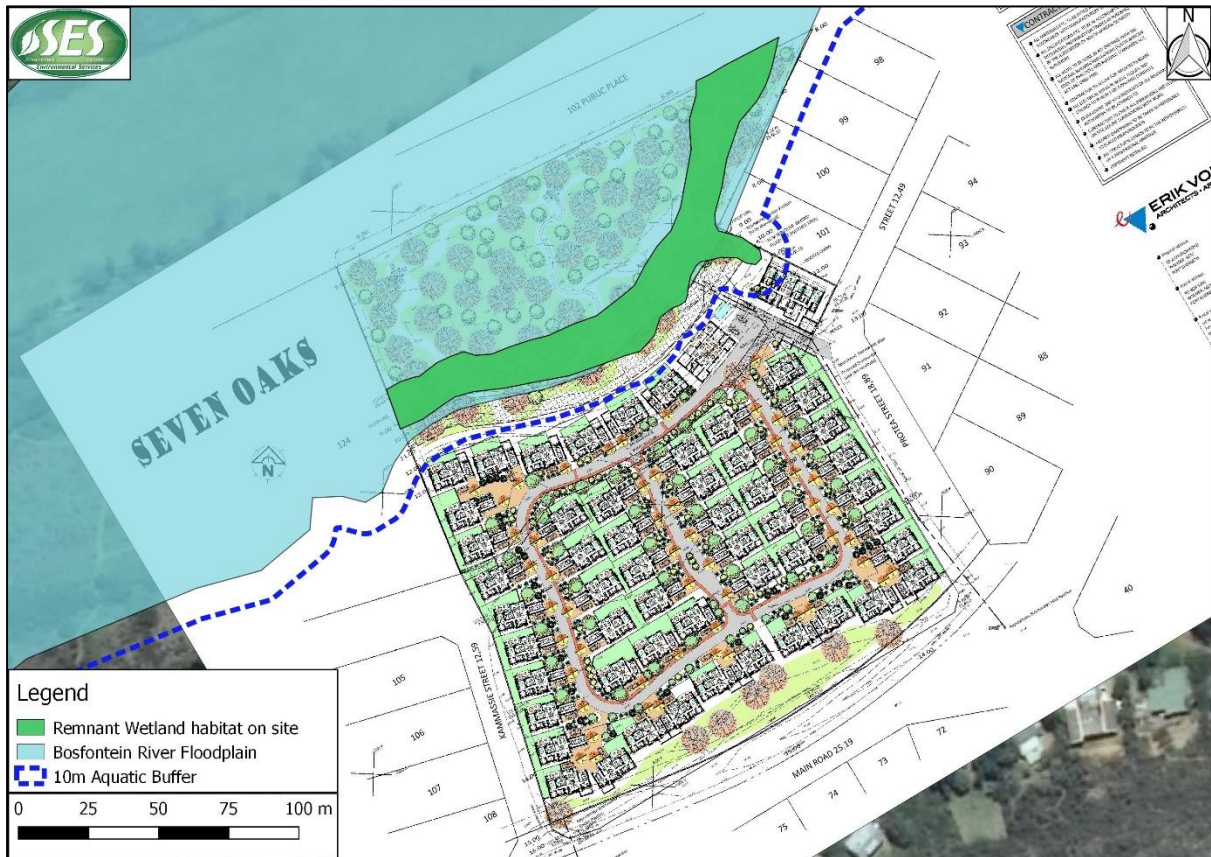
Figure 24: A map showing the recommended 10m buffer from aquatic habitat overlaid on the amended proposed layout: Alternative B
