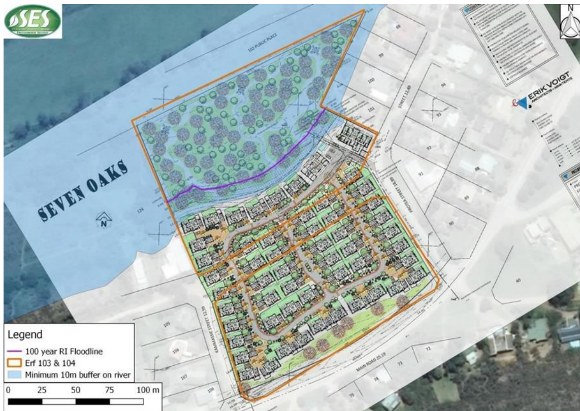
Figure 14: A map showing the recommended 10m buffer from aquatic habitat overlaid on the amended proposed layout.
