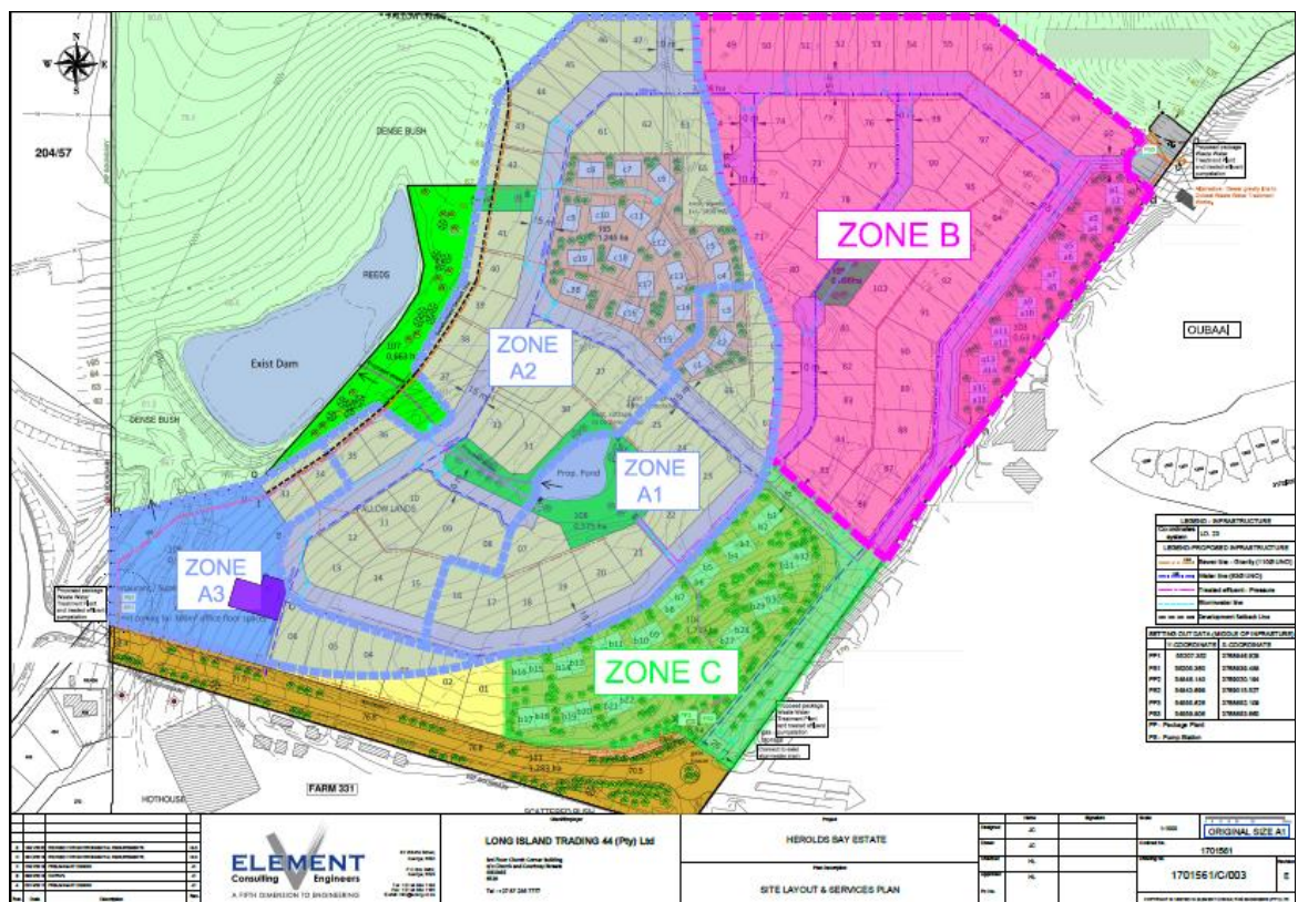
Figure 23: Internal stormwater design zones.
