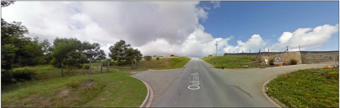
Figure 20: Eastern view along Oubaai Main Road at the proposed access to the filling station (on the left). Sight distance is excellent in both the horizontal and vertical alignments.
