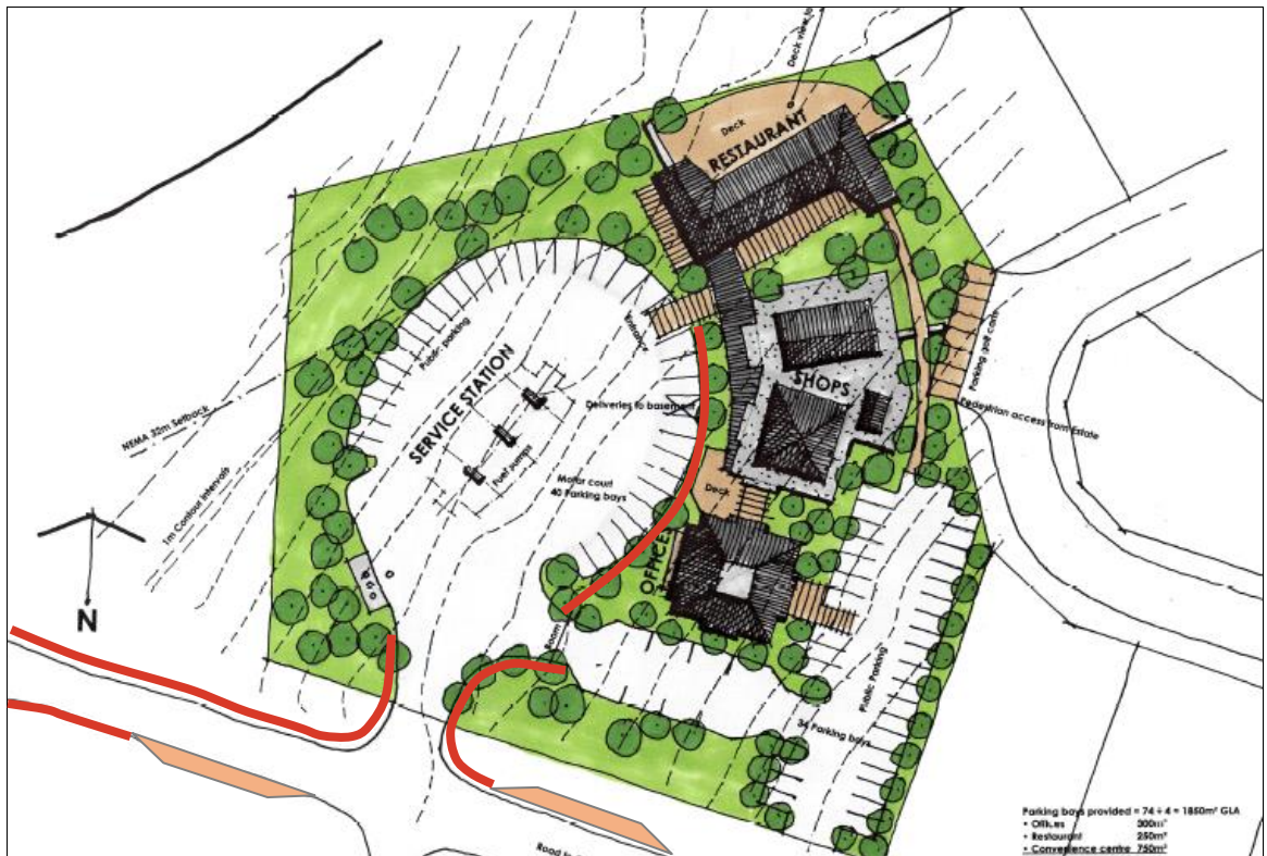
Figure 27: Schematic layout of proposed non-motorized transport facilities (pedestrian walkways) and GIPTN bus stops to be provided at the neighbourhood centre.
