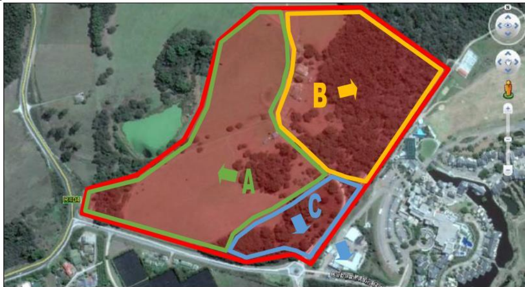
Figure 6: Sewer Drainage Zones (Source: Element Consulting Engineers, 2019)
