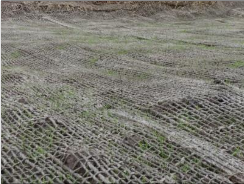
Figure 13: An example of biodegradable netting, such as Bio Jute, for preventing erosion and rehabilitating areas of bare ground.
