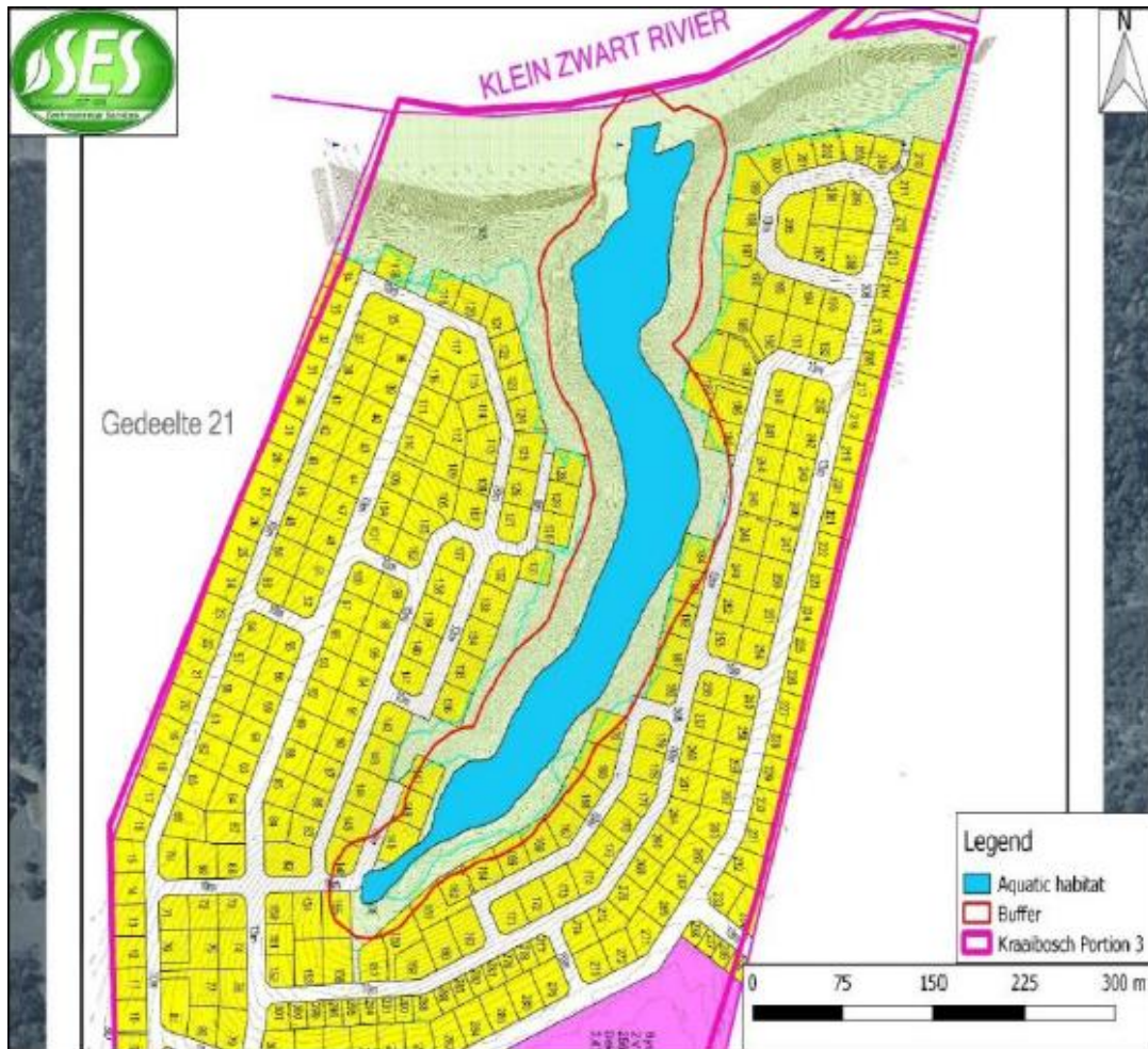
Figure 9: Buffer area surrounding the stream running through the centre of the property
