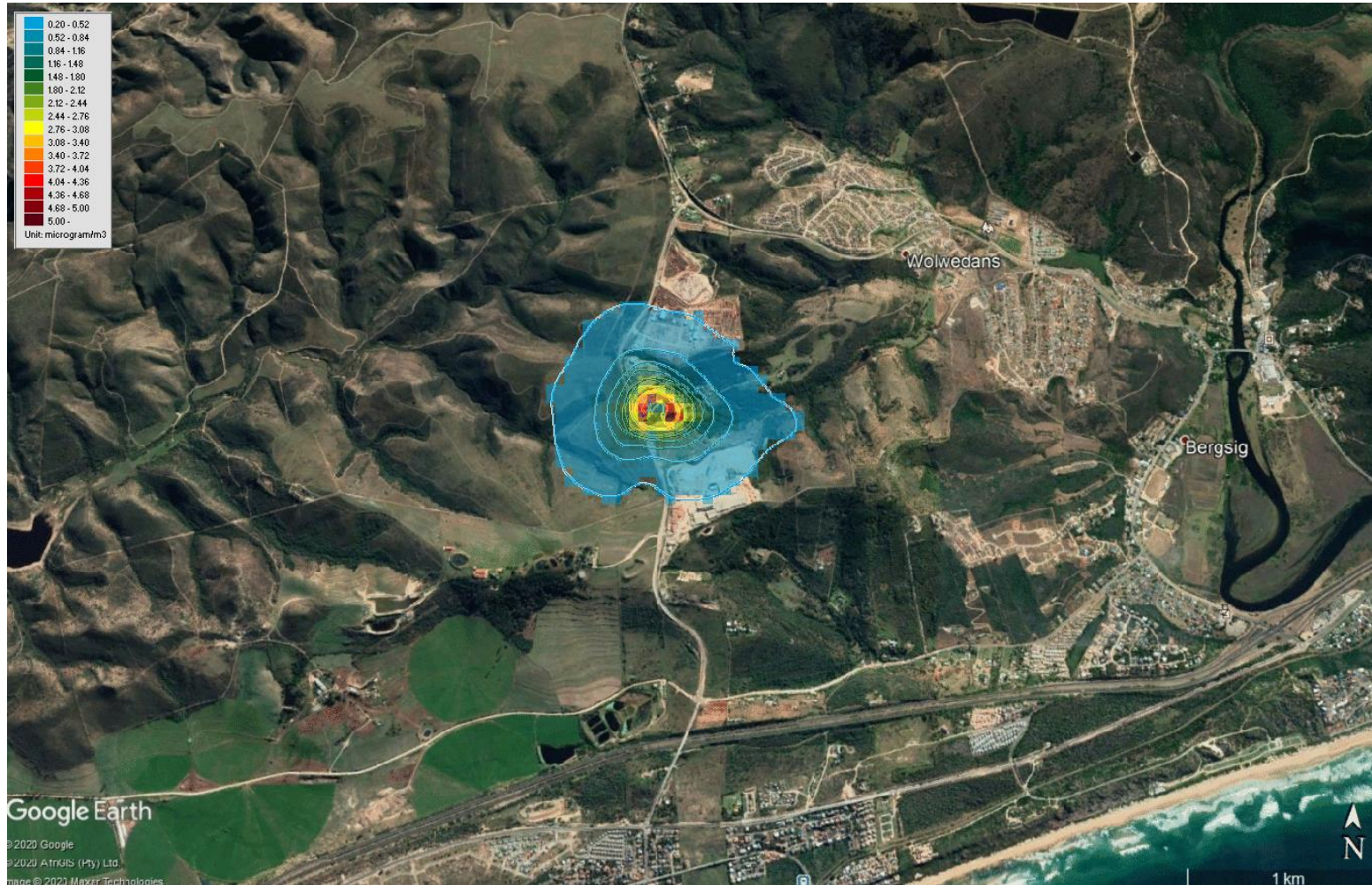
Figure 10: 99-percentile CO Concentrations - Rooikat Operations Only Maximum scale is 5 µg/m 3 . Ambient air quality standard is 30 000 µg/m 3 (30 mg/m 3 )
