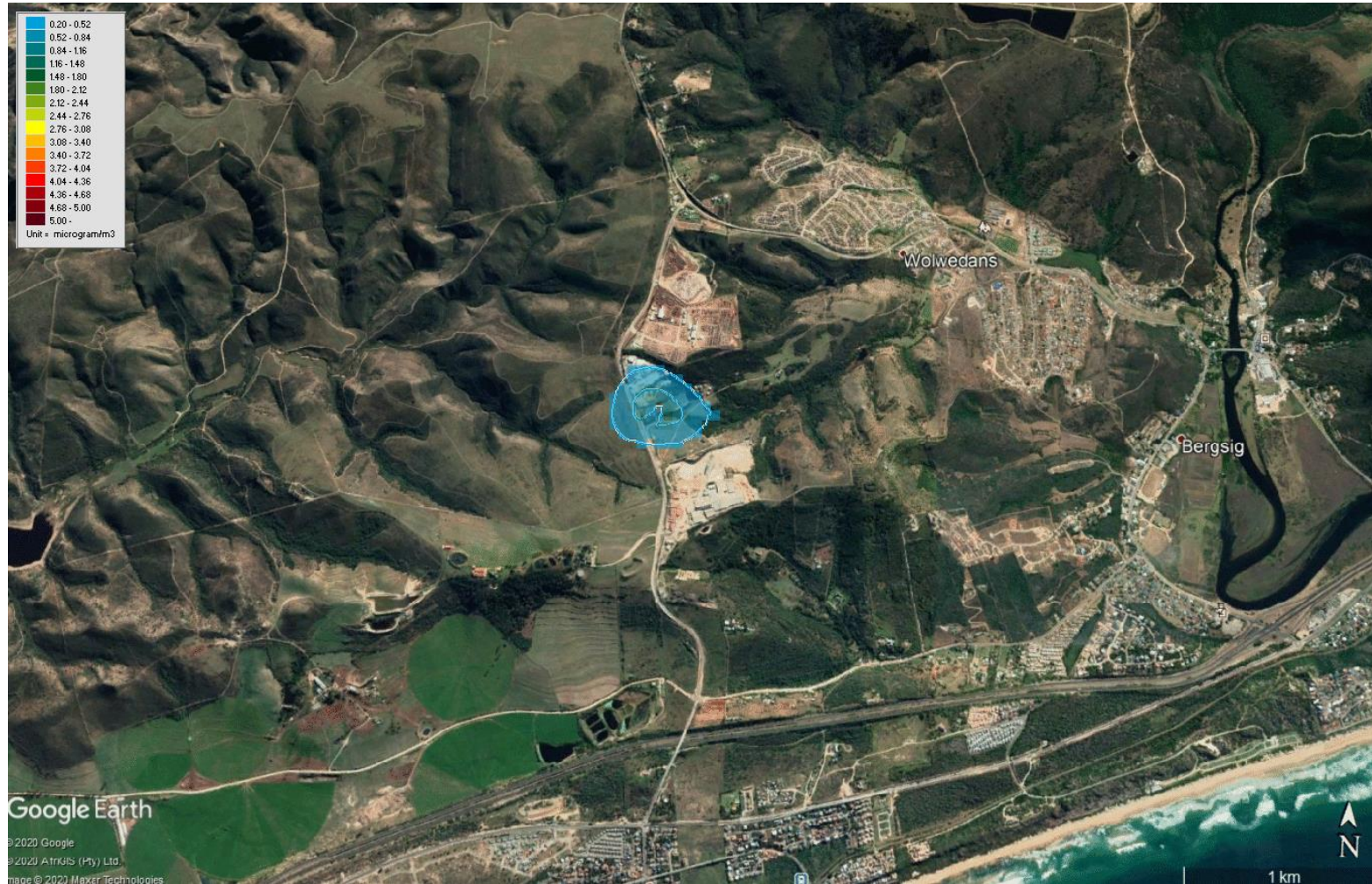
Figure 4: 99-percentile PM10 Daily Averaged Concentrations - Rooikat Operations Only Maximum scale is 5 \mu\text{g}/\text{m}^3 . Ambient air quality standard is 75 \mu\text{g}/\text{m}^3
