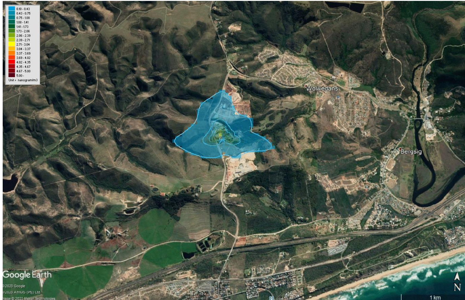
Figure 12: Annual Pb Concentrations - Rooikat Operations Only Maximum scale is 5 ng/m 3 . Ambient air quality standard is 500 ng/m 3 (0.5 µg/m 3 )
