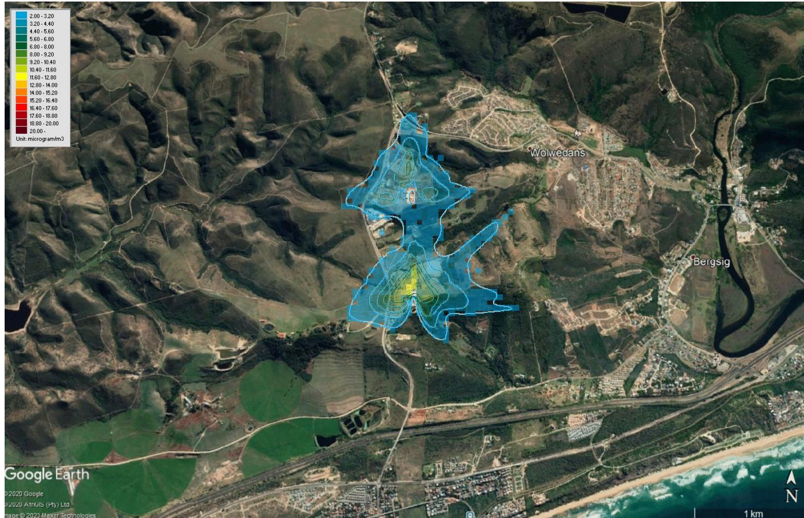
Figure 14: 99-percentile PM10 Daily Averaged Concentrations - Cumulative Sources Maximum scale is 20 µg/m 3 . Ambient air quality standard is 75 µg/m 3
