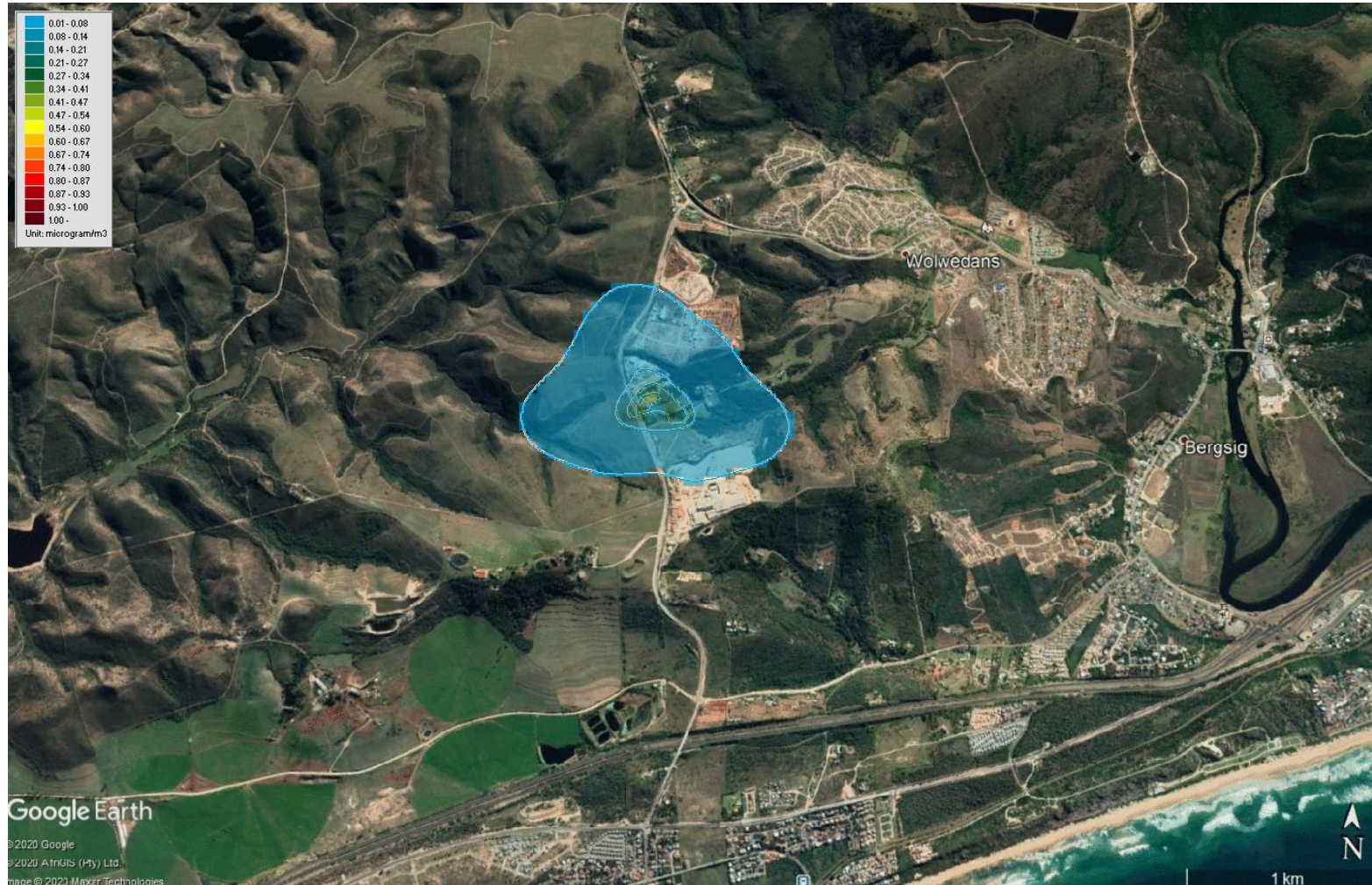
Figure 9: 8-hour Average CO Concentrations - Rooikat Operations Only Maximum scale is 1 µg/m 3 . Ambient air quality standard is 10 000 µg/m 3 (10 mg/m 3 )
