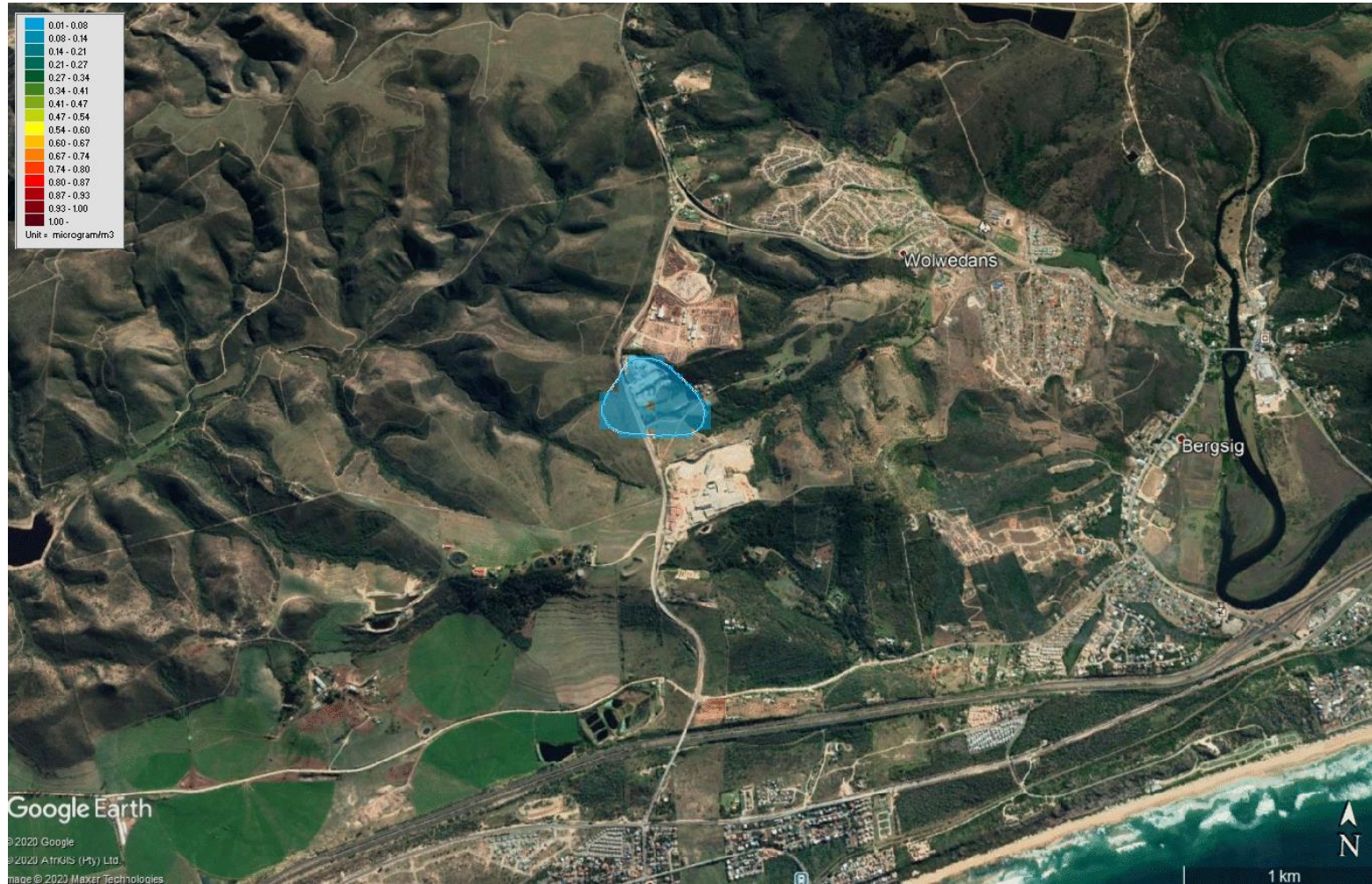
Figure 12: Annual Average C 6 H 6 Concentrations - Rooikat Operations Only Maximum scale is 1 ng/m 3 . Ambient air quality standard is 5 000 ng/m 3 (5 µg/m 3 )
