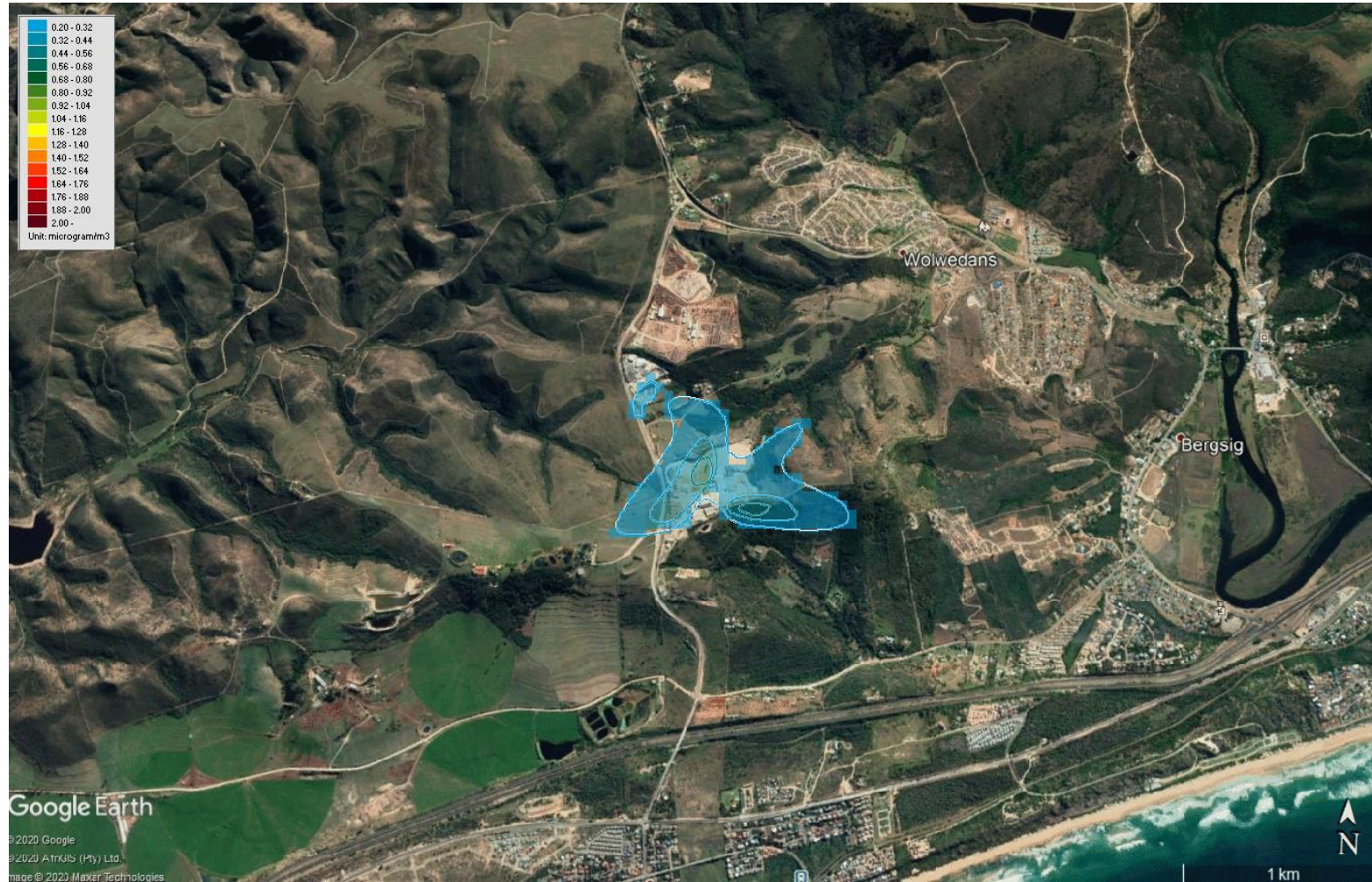
Figure 15: Annual Average SO 2 Concentrations - Cumulative Sources Maximum scale is 2 µg/m 3 . Ambient air quality standard is 50 µg/m 3
