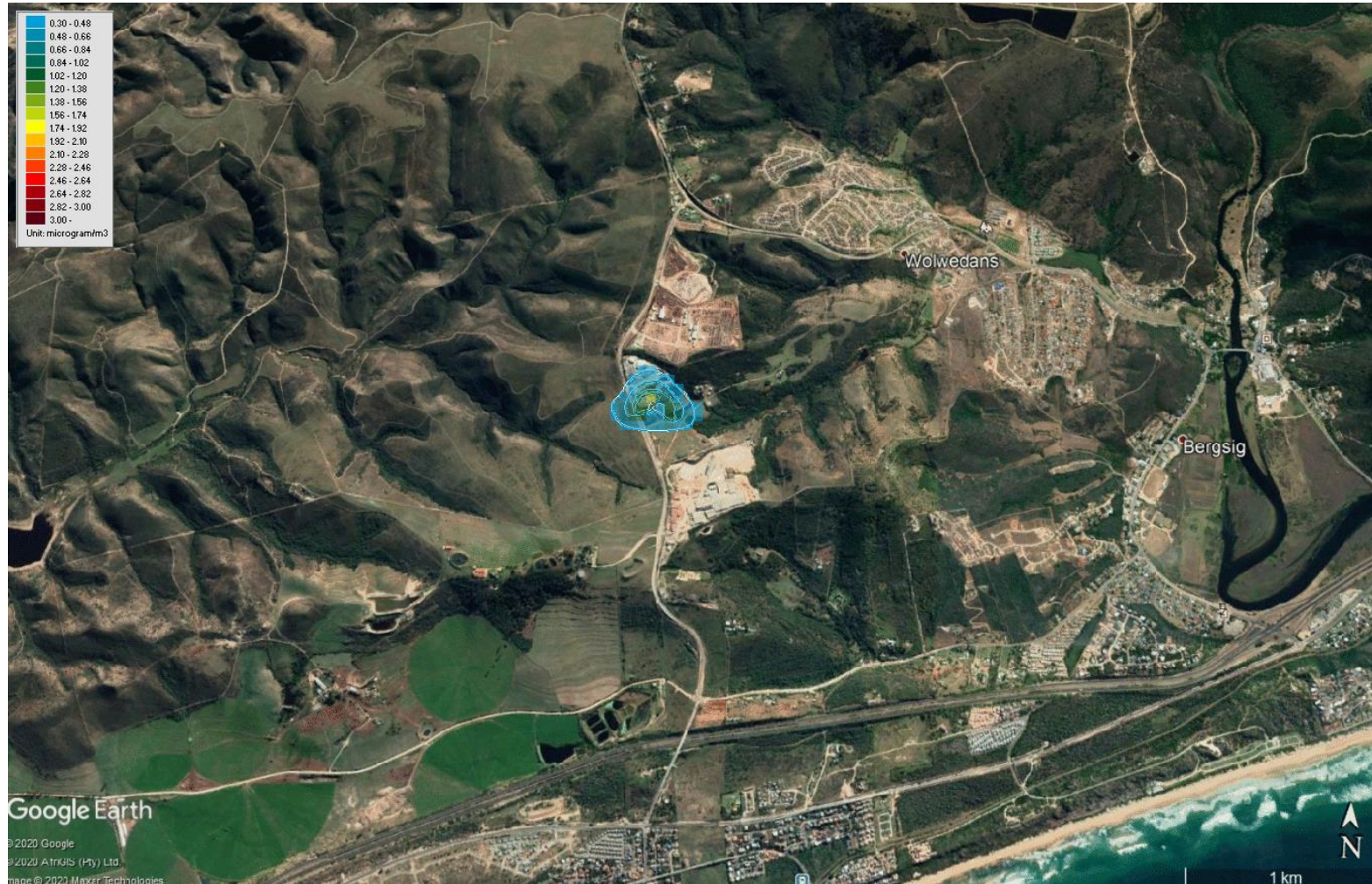
Figure 7: Annual Average NO 2 Concentrations - Rooikat Operations Only Maximum scale is 3 µg/m 3 . Ambient air quality standard is 40 µg/m 3
