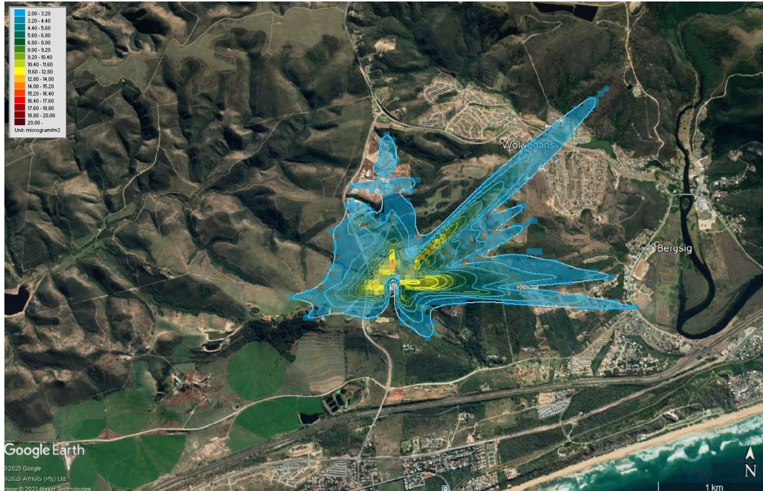
Figure 16: 99-percentile SO 2 Concentrations - Cumulative Sources Maximum scale is 20 µg/m 3 . Ambient air quality standard is 350 µg/m 3
