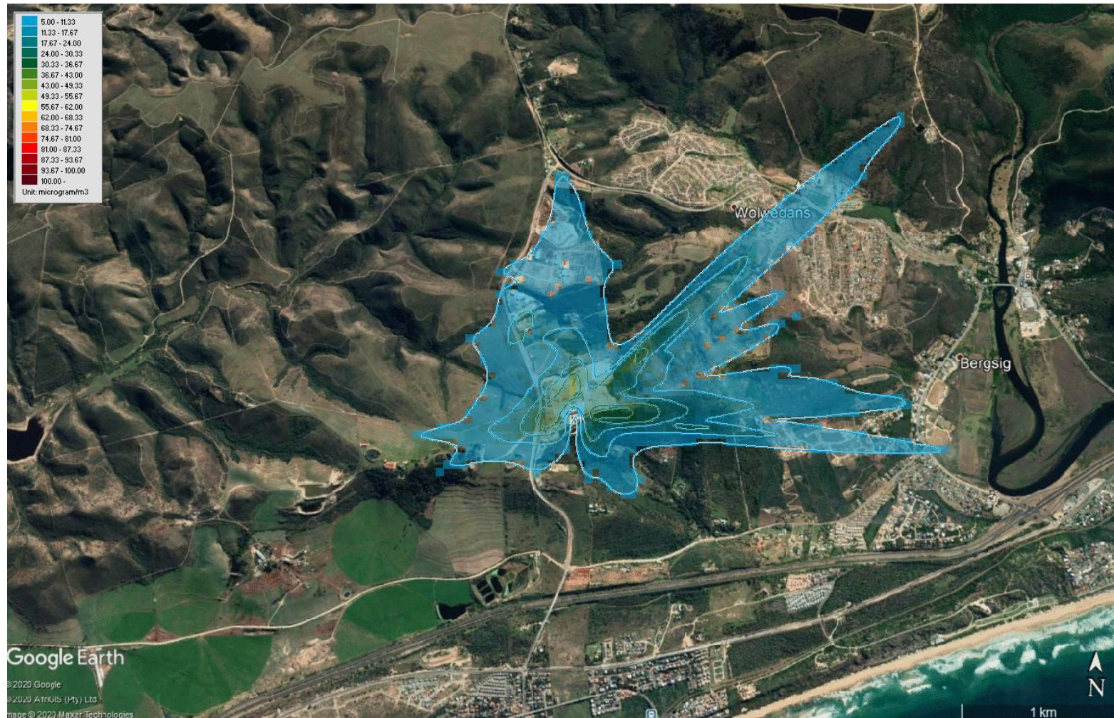
Figure 18: 99-percentile NO 2 Concentrations - Cumulative Sources Maximum scale is 100 µg/m 3 . Ambient air quality standard is 200 µg/m 3
