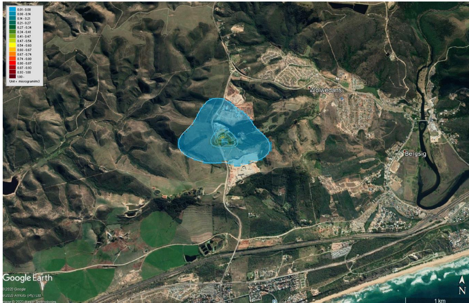
Figure 5: Annual Average SO 2 Concentrations - Rooikat Operations Only Maximum scale is 1 µg/m 3 . Ambient air quality standard is 50 µg/m 3
