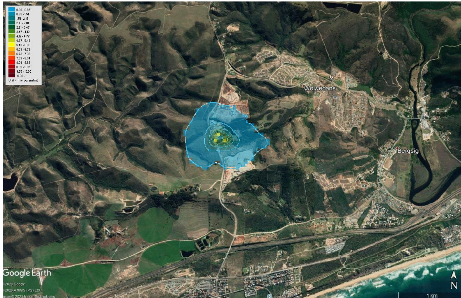
Figure 6: 99-percentile SO 2 Concentrations - Roikat Operations Only Maximum scale is 10 µg/m 3 . Ambient air quality standard is 350 µg/m 3
