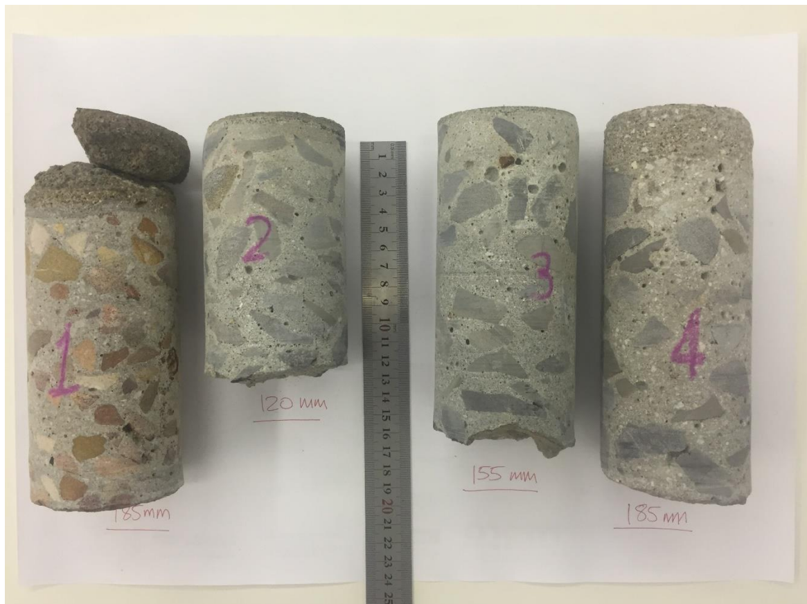
Photo 1: Concrete cores from floor slabs on the ground.
