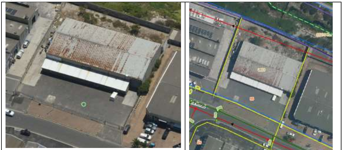
FIGURE 2: Erf 2433, MGI: Aerial view and Plan viewer [with Water (blue), Sewer (red) and Stormwater (green) services location in relation to the erf boundaries]
