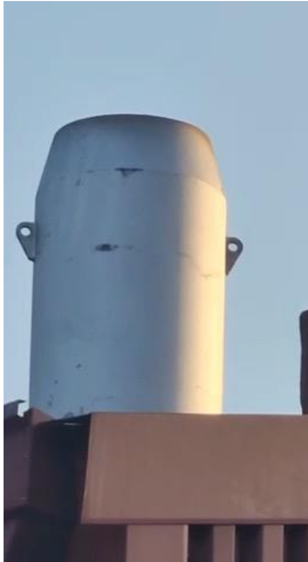
Figure 9: No visible emissions can be seen at a primary temperature of 562 °C and secondary temperature of 818 °C.
