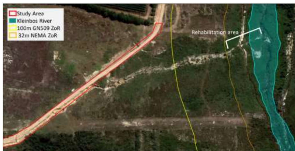
Figure 21: Area to be rehabilitated by infilling the shallow gully/flow path with the deposited sediment and revegetating the area.
