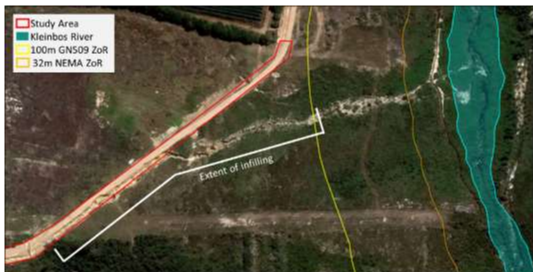
Figure 19: The length of erosion gully proposed to be infilled with rip-rap, as per the engineering drawing (Figure 3) relative to the Kleinbos River and the 100m GN509 ZoR.
