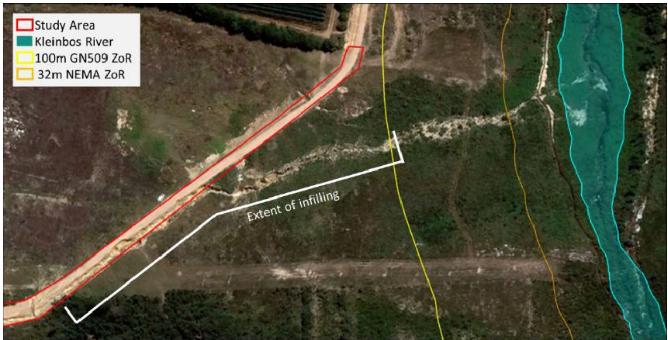
Figure 4: The length of erosion gully proposed to be infilled with riprap, as per the engineering drawing relative to the Kleinbos River and the 100m GN509 ZoR.
