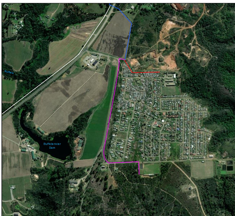
Figure 9: The 315mm uPVC splits into a proposed 200mm UPVC Supply Pipeline to Kurland Housing 562 (pink polyline) and 200mm UPVC Supply Pipeline to Kurland Township (red polyline).
