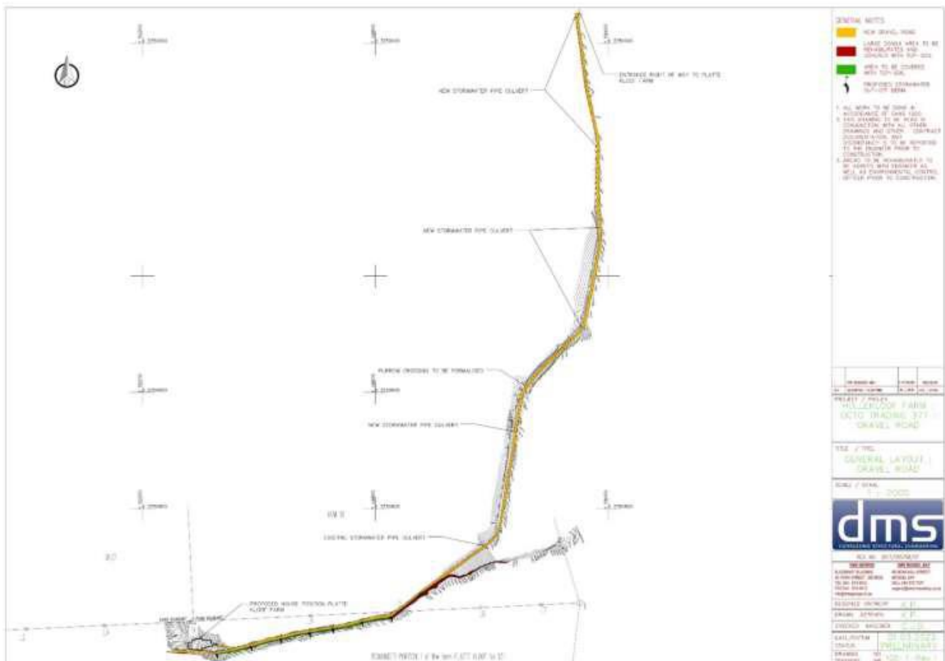
Figure 14: Proposed remediation actions for the erosion gully (donga – green and red) along the access road (yellow), as provided by DMS Consulting Structural Engineering (March 2022). Note that stormwater cut-off berms will be installed in the erosion gully section along the southern portion of the road (green). The gully will be infilled for the section it diverts from the road (red) toward the Kleinbos River (blue dashed line) in the east. (Figure 3 of the Freshwater Assessment)
