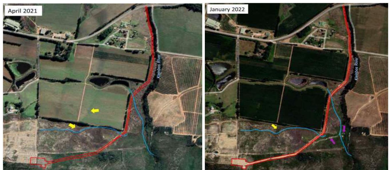
Figure 17: Digital satellite imagery depicting the locality of the study area (red outline) prior to the construction activities (2021) and after (2022). Furrows (white dashed lines) drain surface runoff and water from the Kleinbos River. Faint signatures (yellow arrows) associated with potential small drainage lines are evident north of the study area. An erosion gully (pink arrows) is noticeable, diverting away from the access road to the Kleinbos River. (Figure 8 of the Freshwater Assessment)
