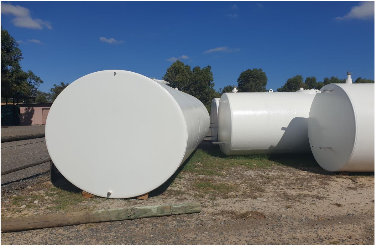
Photo 3: 8 x23m 3 above ground storage tanks which are not in use are stored on the property. tanks are also being refurbished on the property.
