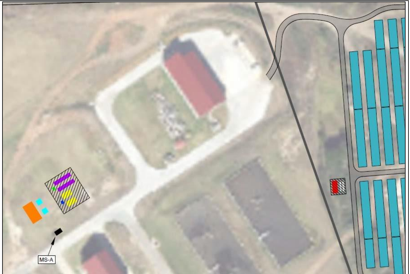
Figure 14: Substation (orange), MV Solar station (red) and Battery/generator station (purple and yellow)
