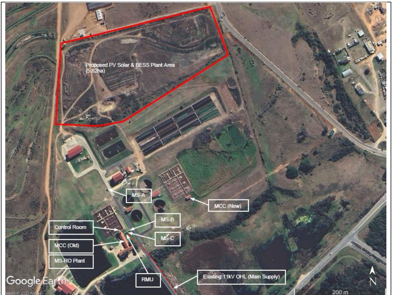
Figure 1: Site Layout: Hartenbos WWTW (Existing)
