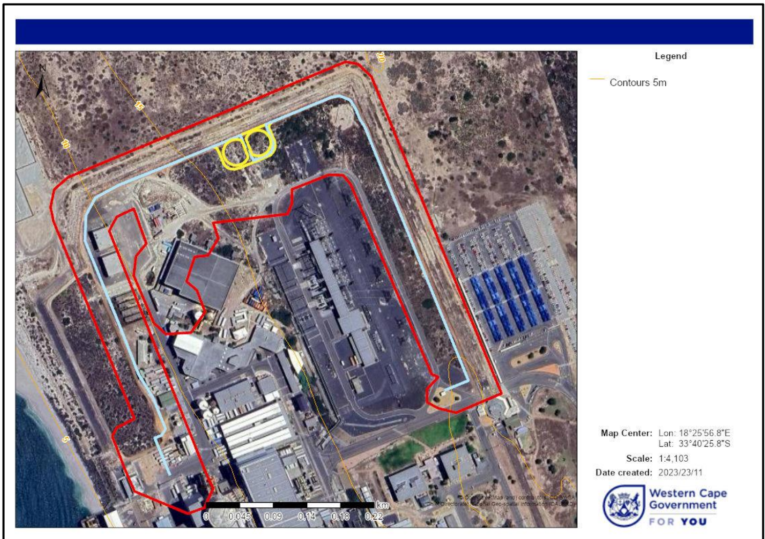
Figure 4 Topology of the study area showing 5 meter contour lines (Red polygon = Study area, Yellow polygons = Proposed reservoirs, Blue lines = Proposed pipelines; map generated in Cape Farm Mapper version 3, Western Cape Department of Agriculture).
