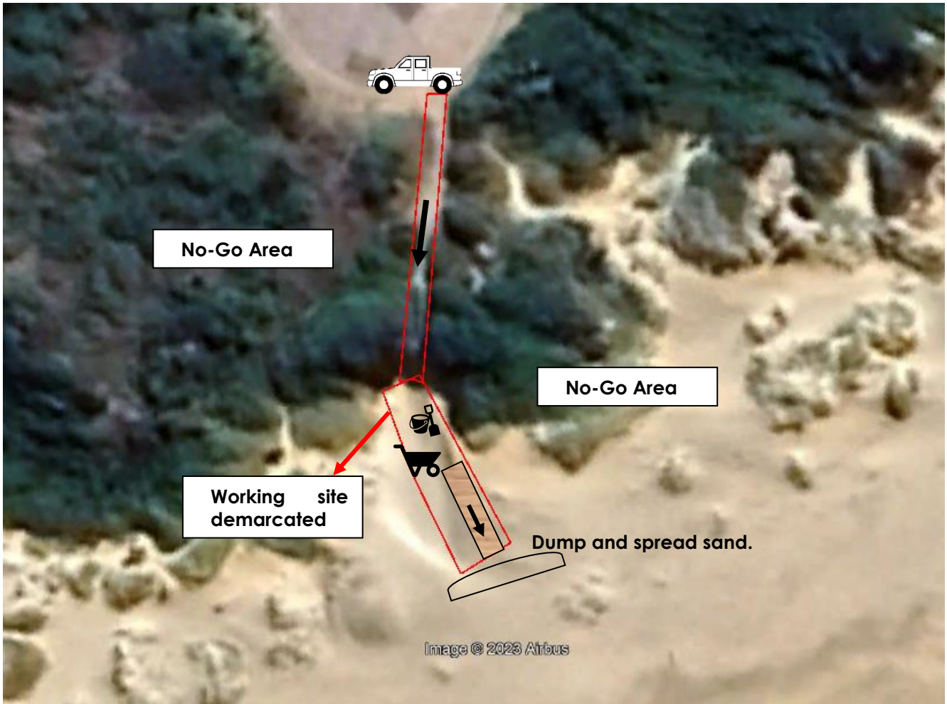
Figure 14: Illustration of maintenance by hand at Sump 2.
