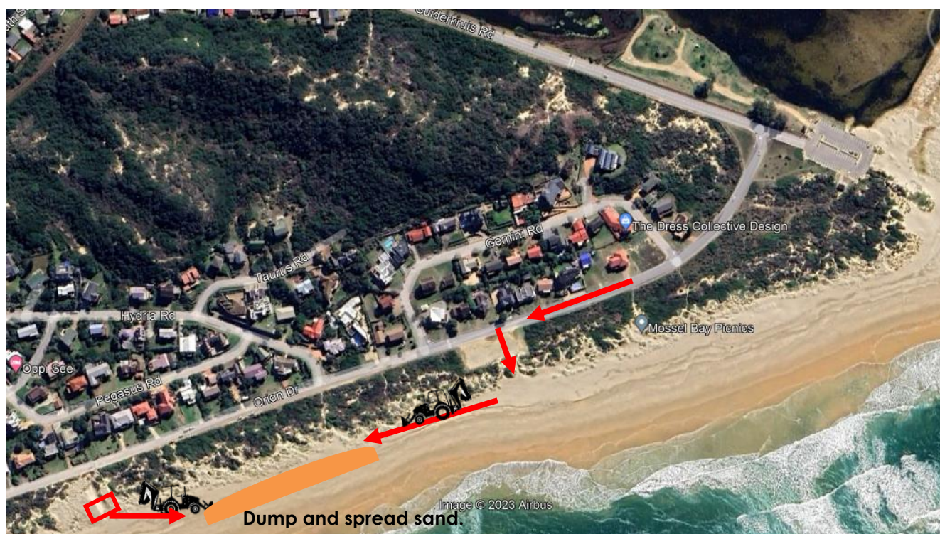
Figure 19: Alternative entry point for the TLB from parking area as indicated.
