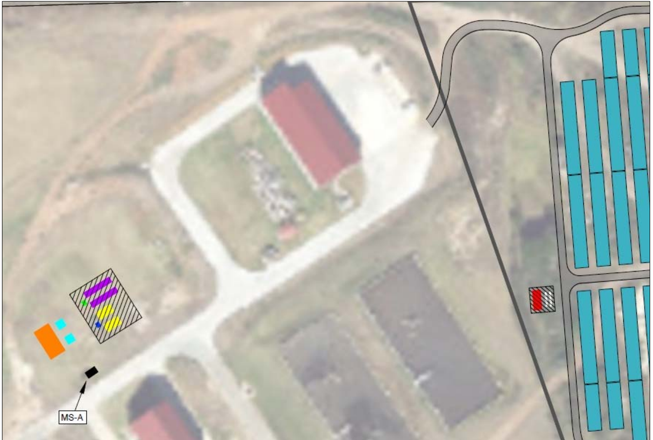
Figure 5-8: Substation (orange), MV Solar station (red) and Battery/generator station (purple and yellow)
