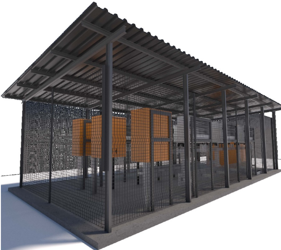
Figure 4-13: Typical String Inverter Canopy (Credit: Eversolar)
