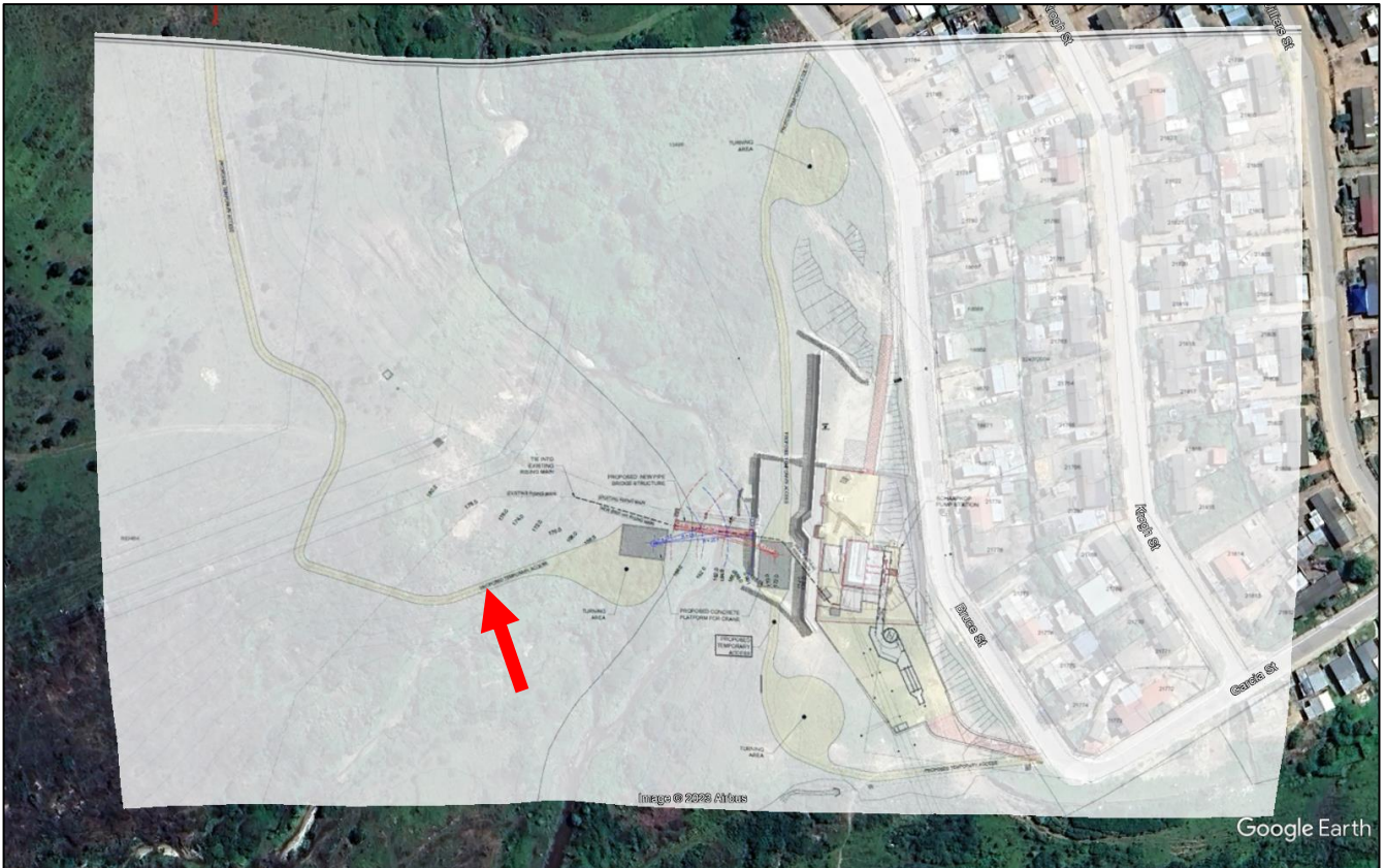
Figure 9: Temporary work areas and proposed gravel road down to the pipe bridge
