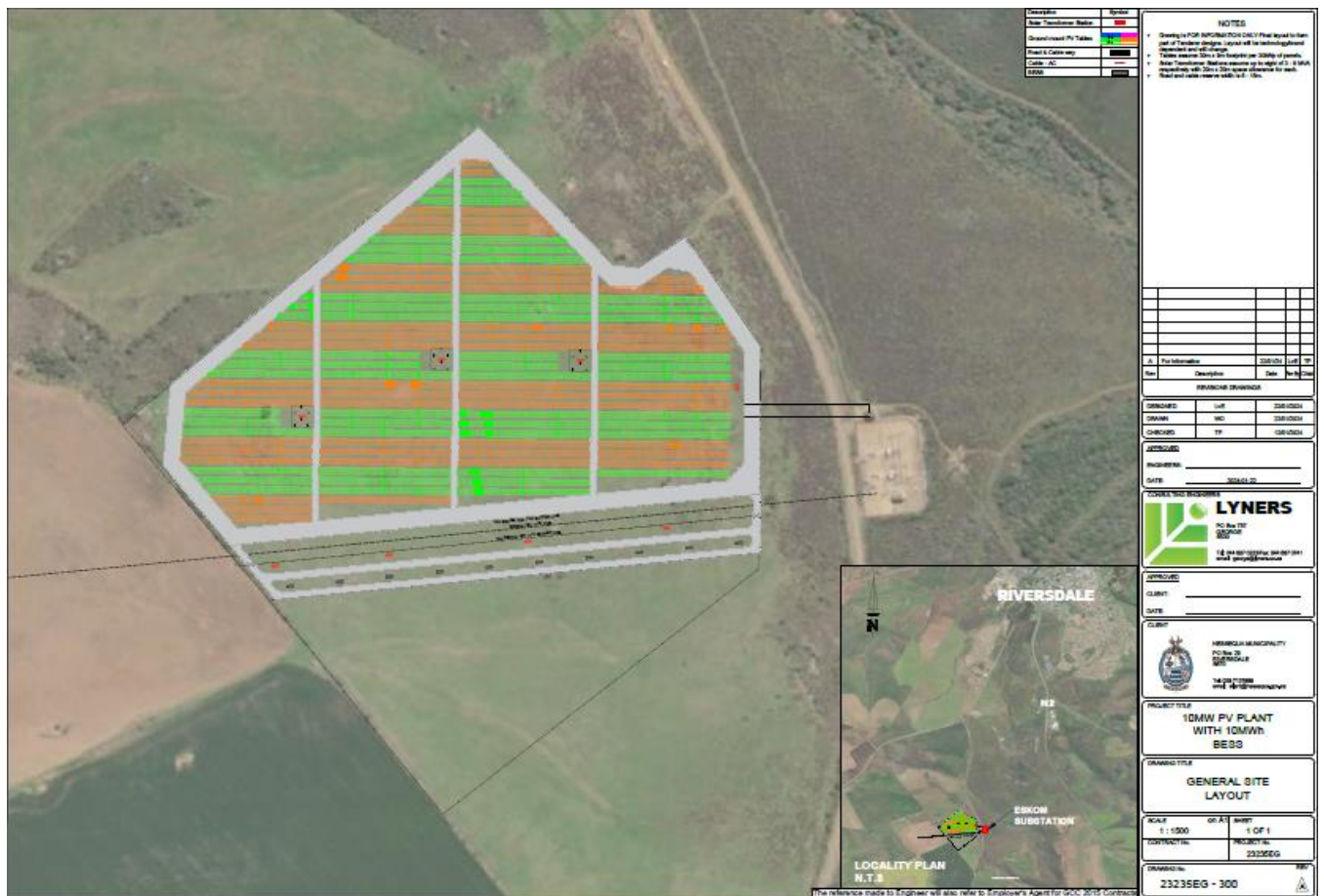
Figure 4. Proposed layout of the Riversdale 10MW Solar PV Plant with Battery Energy Storage System
