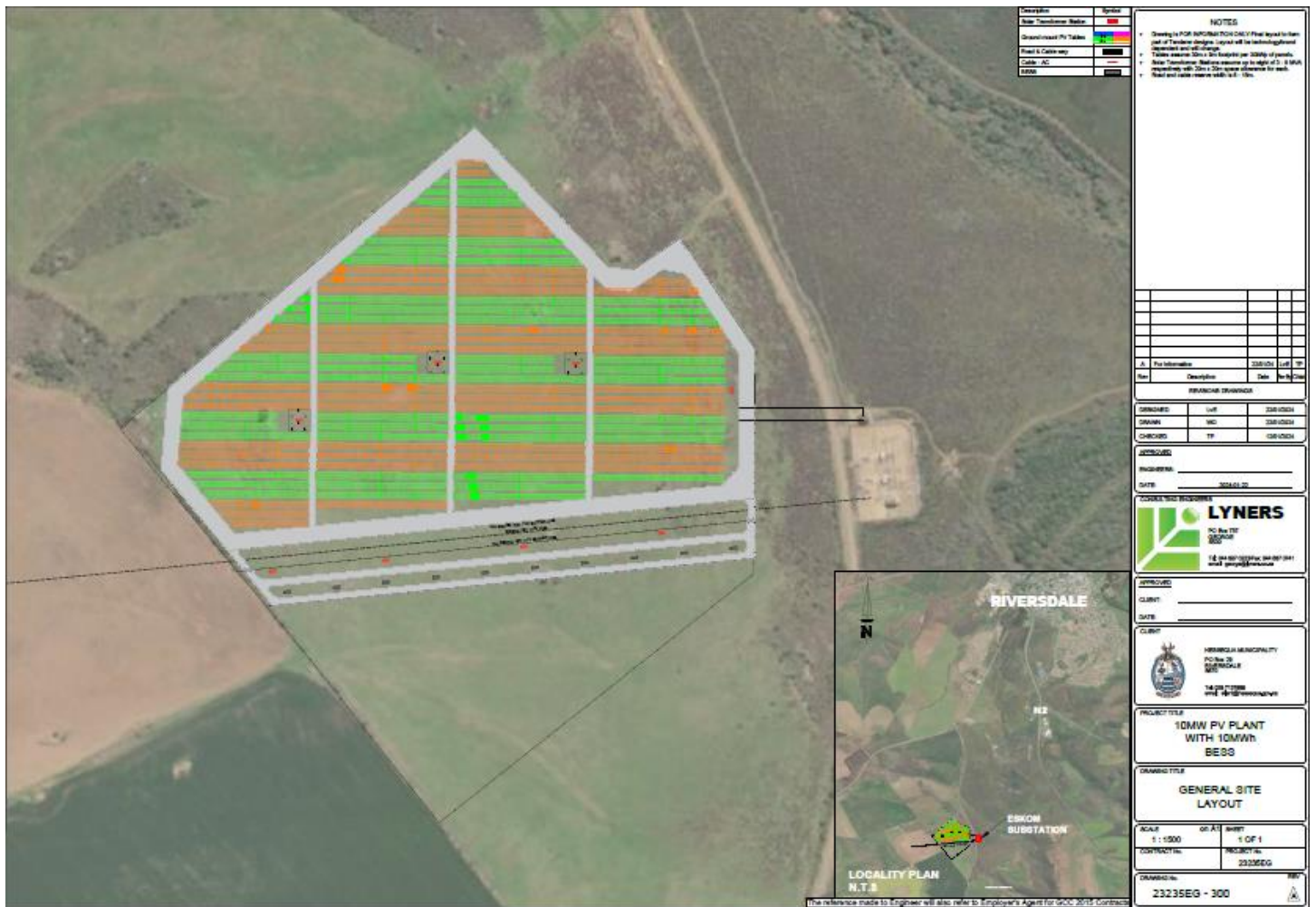
Figure 3. Proposed layout of the Riversdale 10MW Solar PV facility with Battery Energy Storage System
