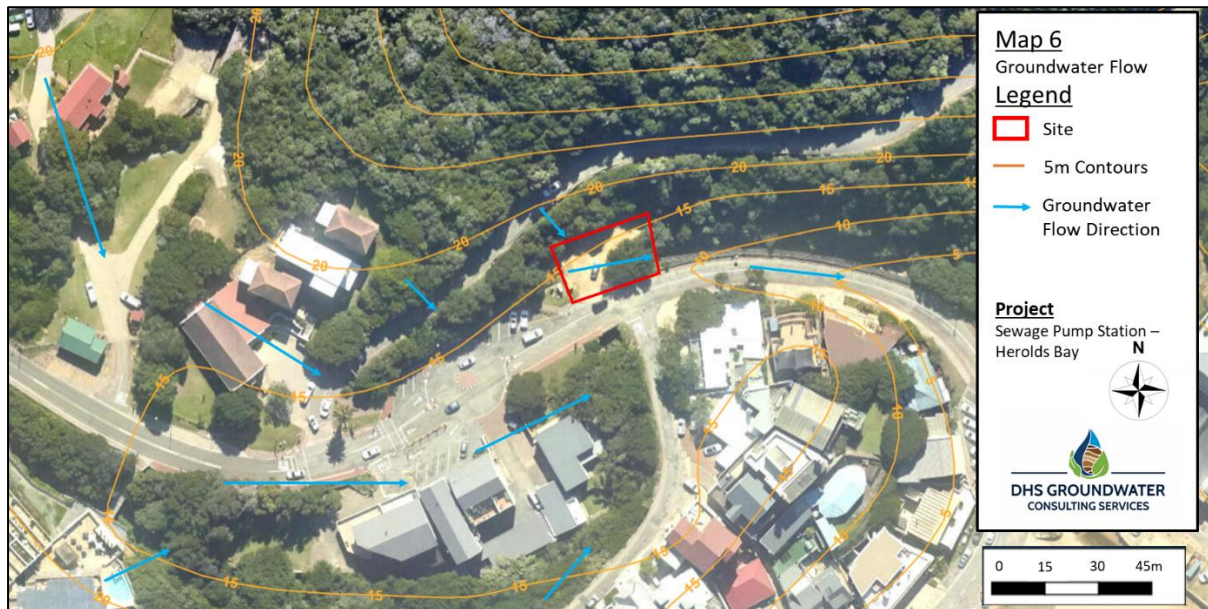
Figure 8. Map with 5m contours showing the inferred groundwater flow direction.
