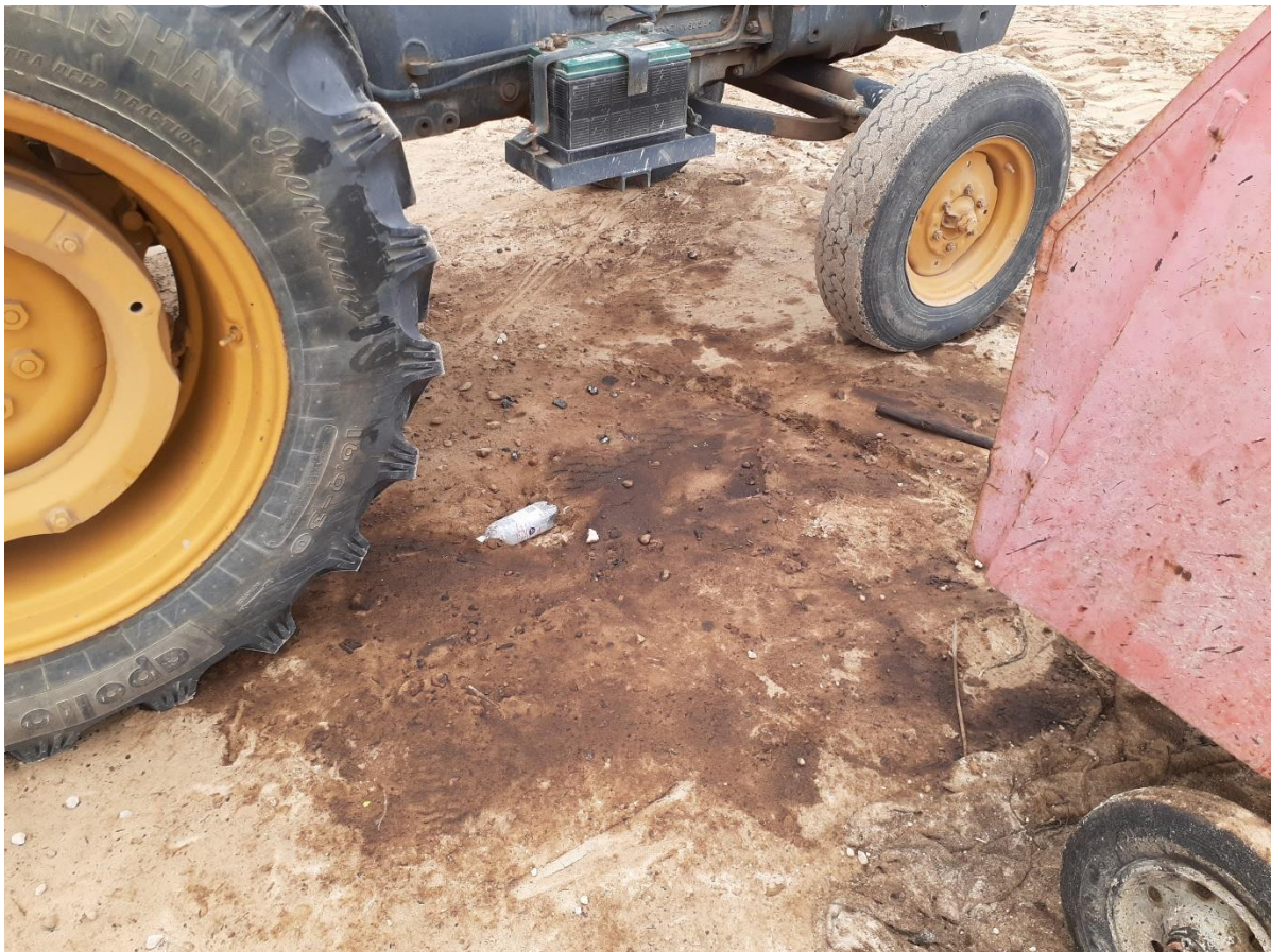
Photo 4: A large diesel spill beneath the tractor was noted on the site. The foreman was informed to pick up the contaminated sand and dispose of it at the Municipal waste disposal facility.
