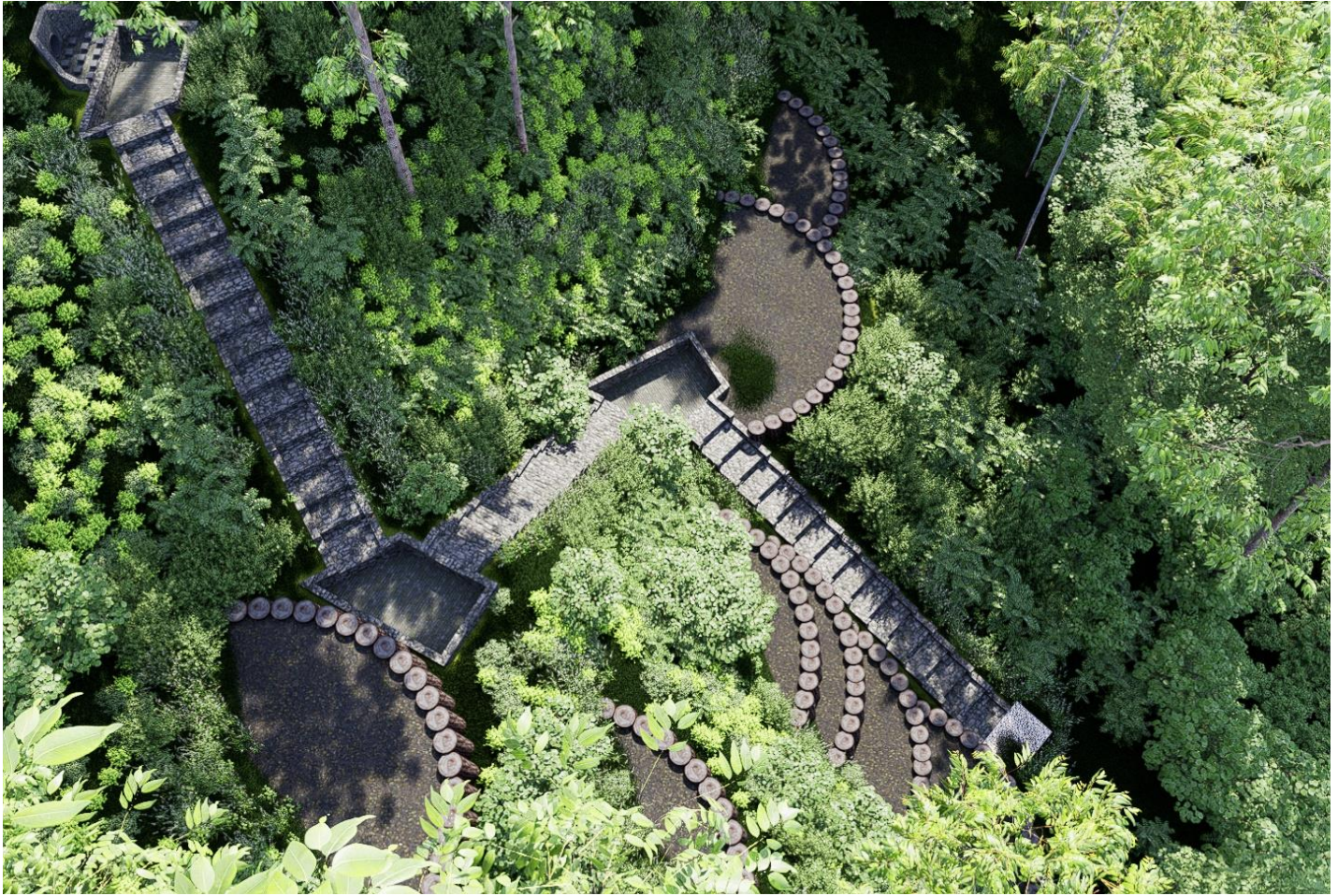
Figure 22 –Elevated top view of the proposed stilling pond and water stair system with discharge over gabion mattress structure at the bottom of the system.
