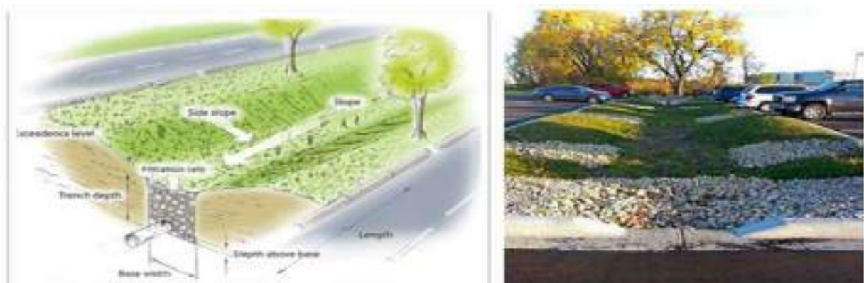
Figure 2-2 - Schematic Representation of Vegetated Swale
