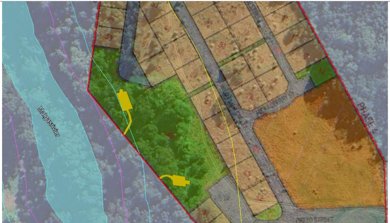
Figure 26: A conceptual layout plan of the original (alternative 1) stormwater structures in the western corner of the property.
