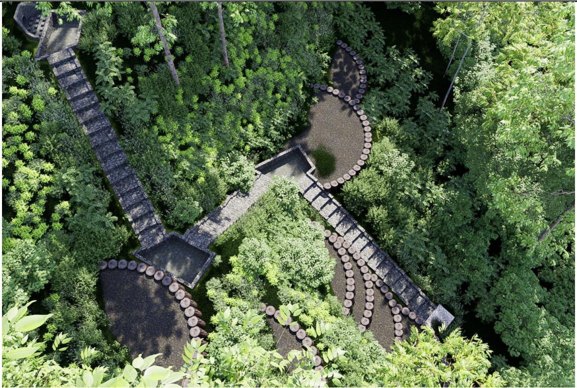
Figure 23: Elevated top view of the proposed stilling pond and water stair system with discharge over gabion mattress structure at the bottom of the system.
