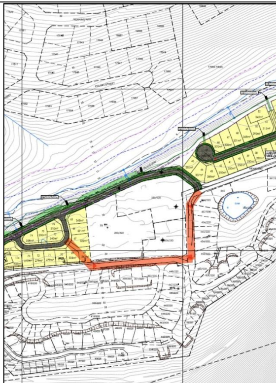
Figure 11: Proposed stormwater layout (Alternative 1)
