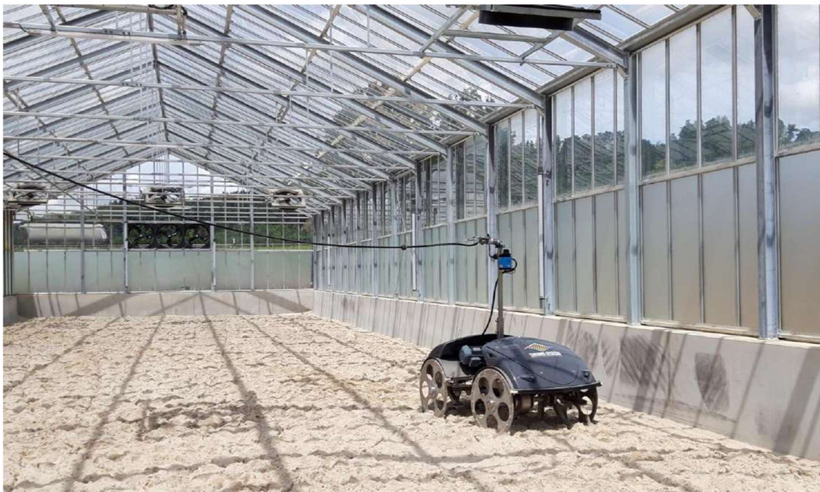
Figure 6-20: Electric mole as part of the SolarBatch system by Thermo-Systems.
