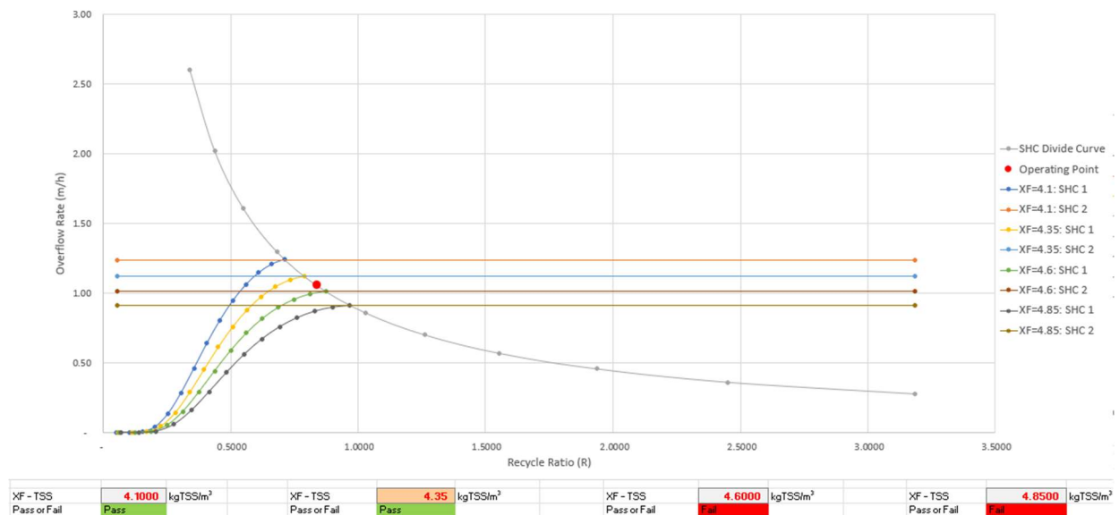
Figure 5-8: Design and Operation chart of SST based on a single reactor with 4x25m Dia. SSTs (UCT settled process)
