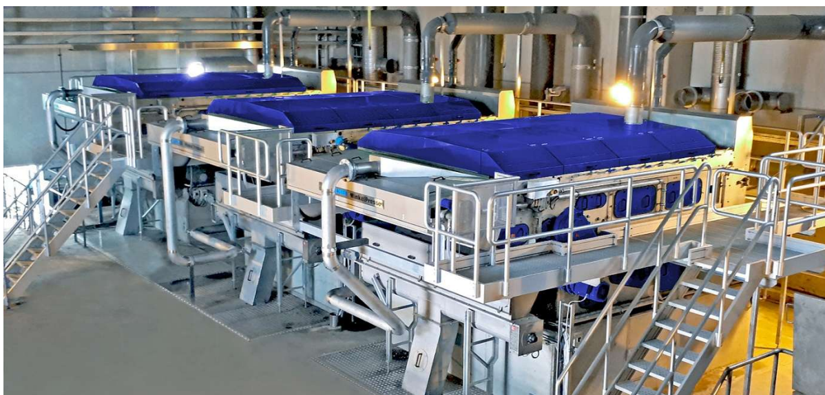
Figure 7-27: Example belt press installation showing 3 filter belt presses
