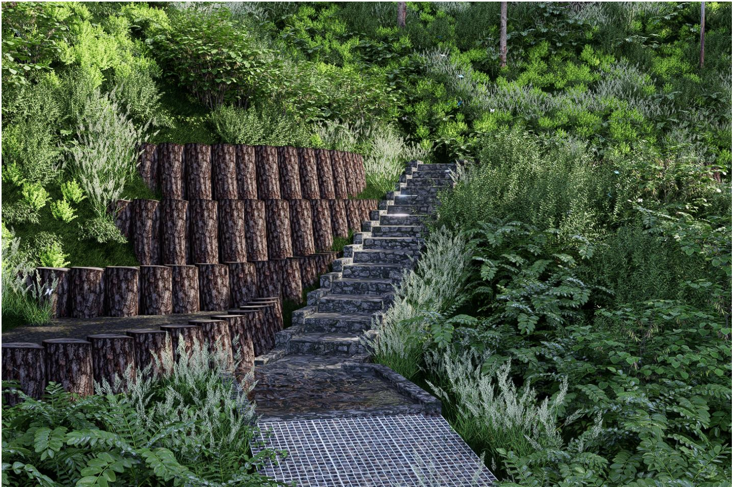
Figure 27 –View of the proposed stilling outflow pond and reno gabion mattress for the discharge. Flow from the cascading structure is halted in the stilling pond before a slow trickle overflow into the gabion mattress.
