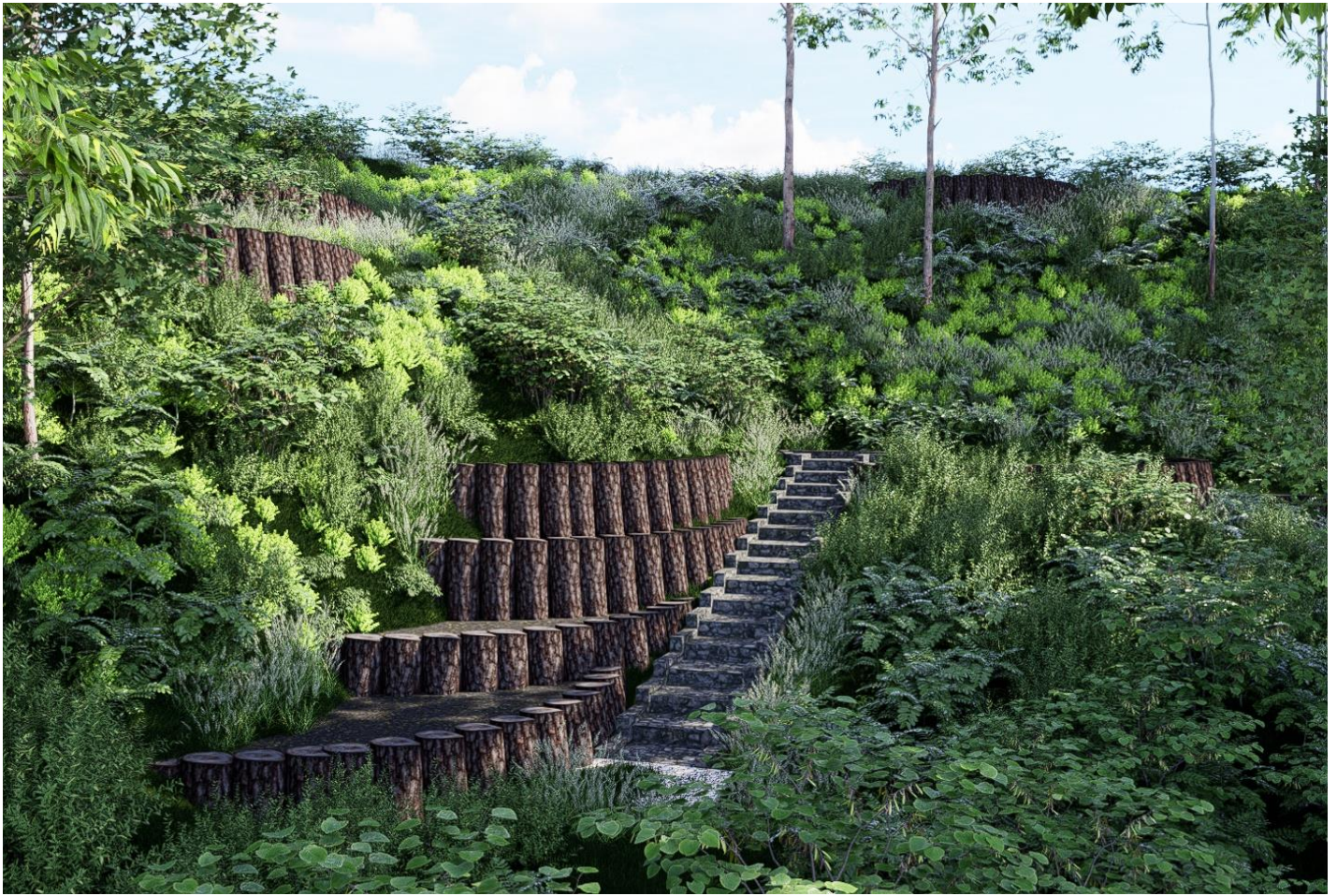
Figure 23 –Side view of the proposed stilling pond and water stair system with discharge following the natural embankment slopes that will be terraced.
