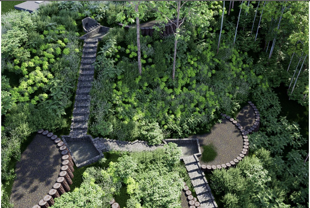
Figure 20: Outflow Headwall structure into 1st stilling pond, followed by 1st water stair section to the 2nd stilling pond.
