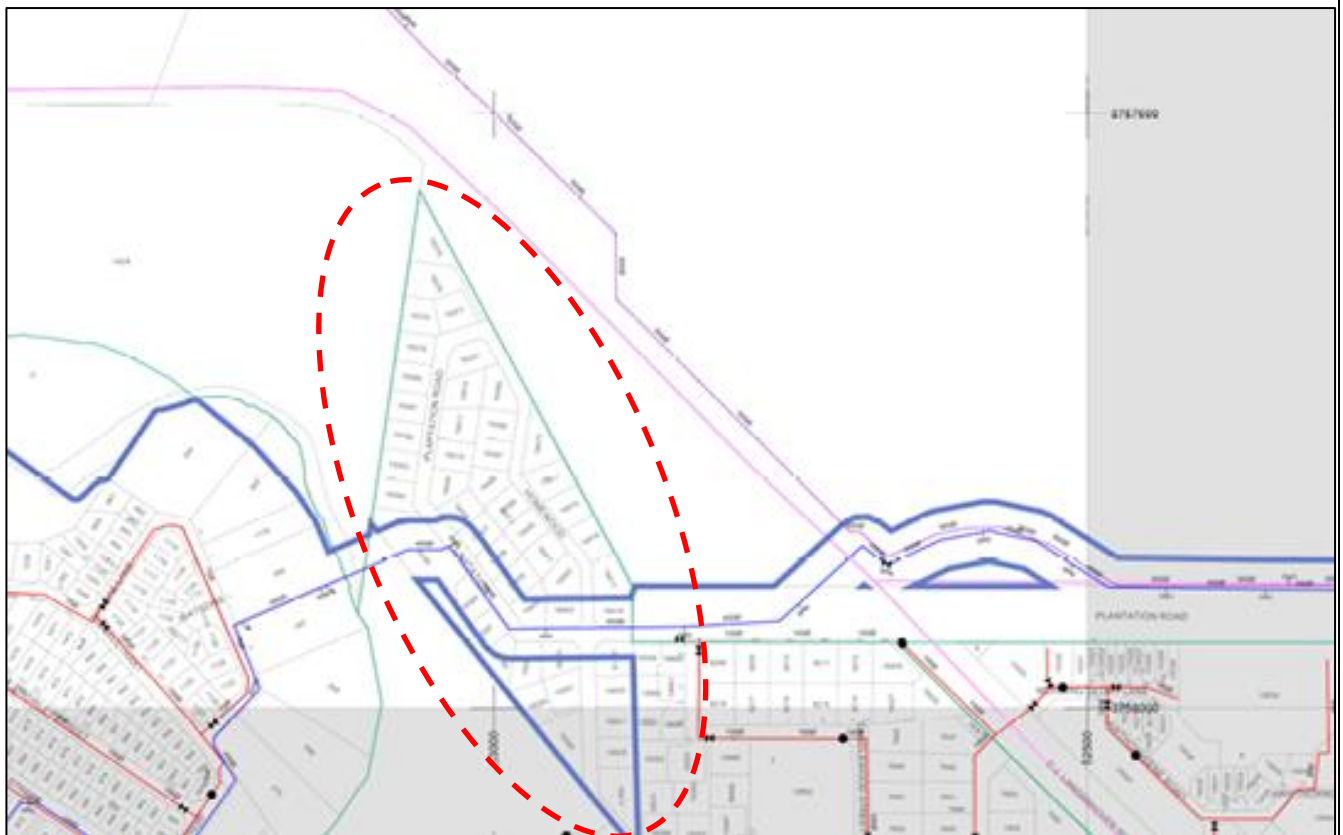
Figure 11: 450mm diameter Municipal Bulk Supply GRP Pipe that runs through the planned development site (red dashed circle).
