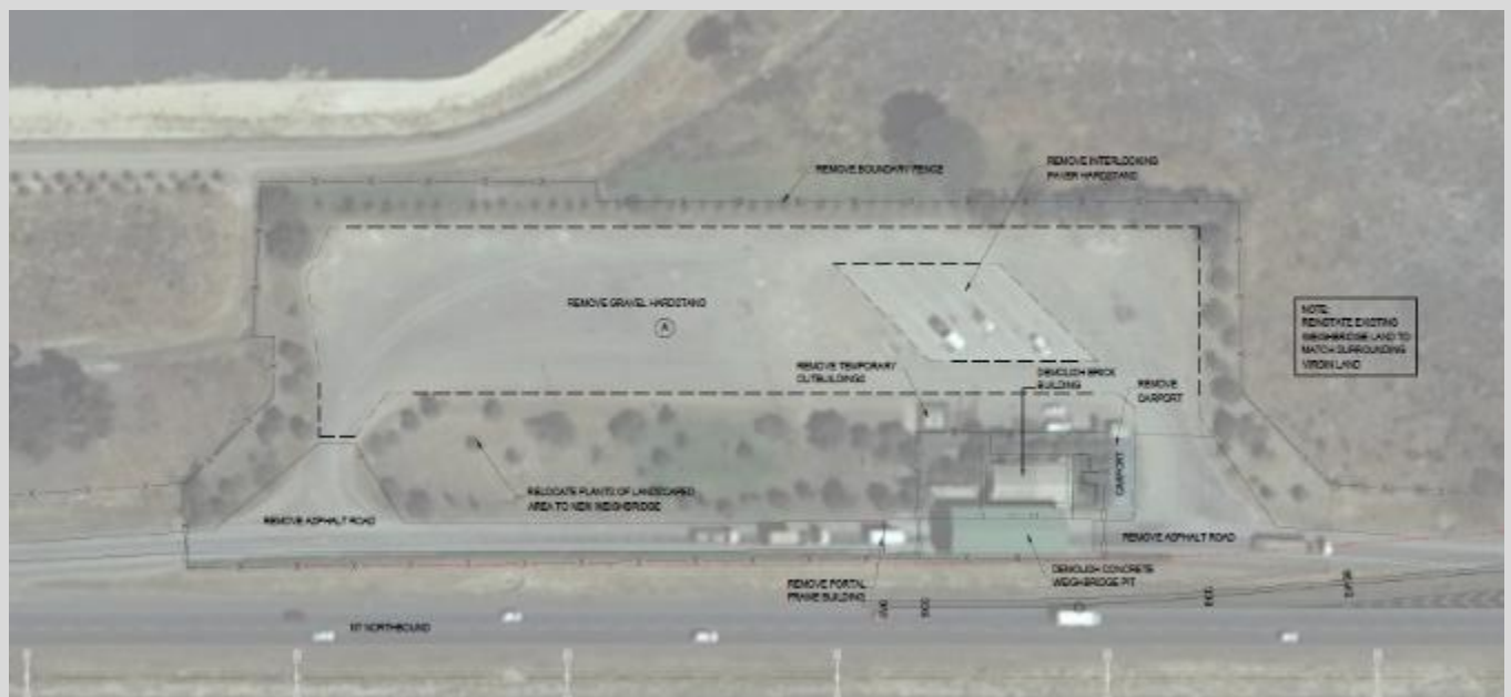
Figure 3. The Demolition plan for the existing weighbridge facility after the new weighbridge is established.
