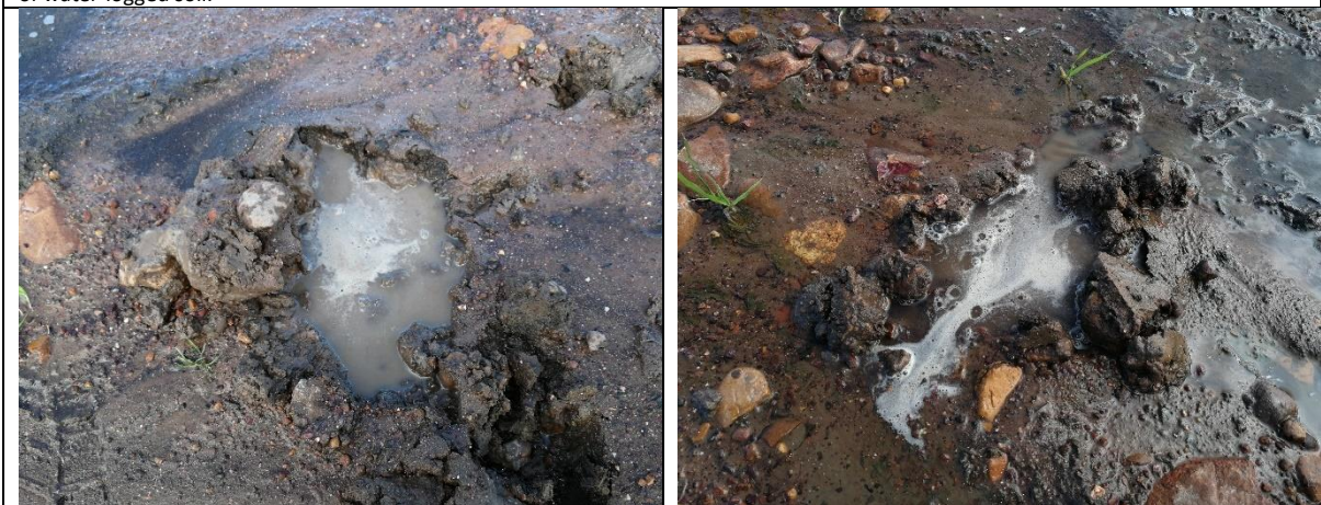
Above: Seasonal Seep Wetland Area soil auger sample drill hole (approximately 30 cm deep) immediately refilling with water indicating water-logged soil due to significant rain events. The seep wetland area is still anticipated to be seasonal.
