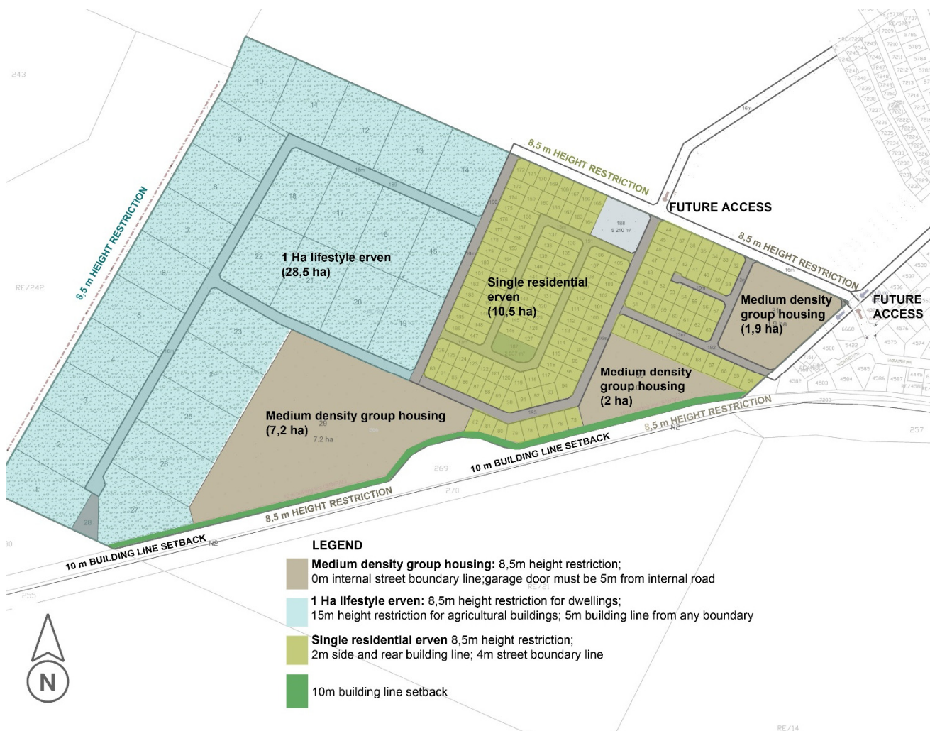
Figure 36: Plan showing building setback lines on site and maximum building heights for the site (not to scale).
