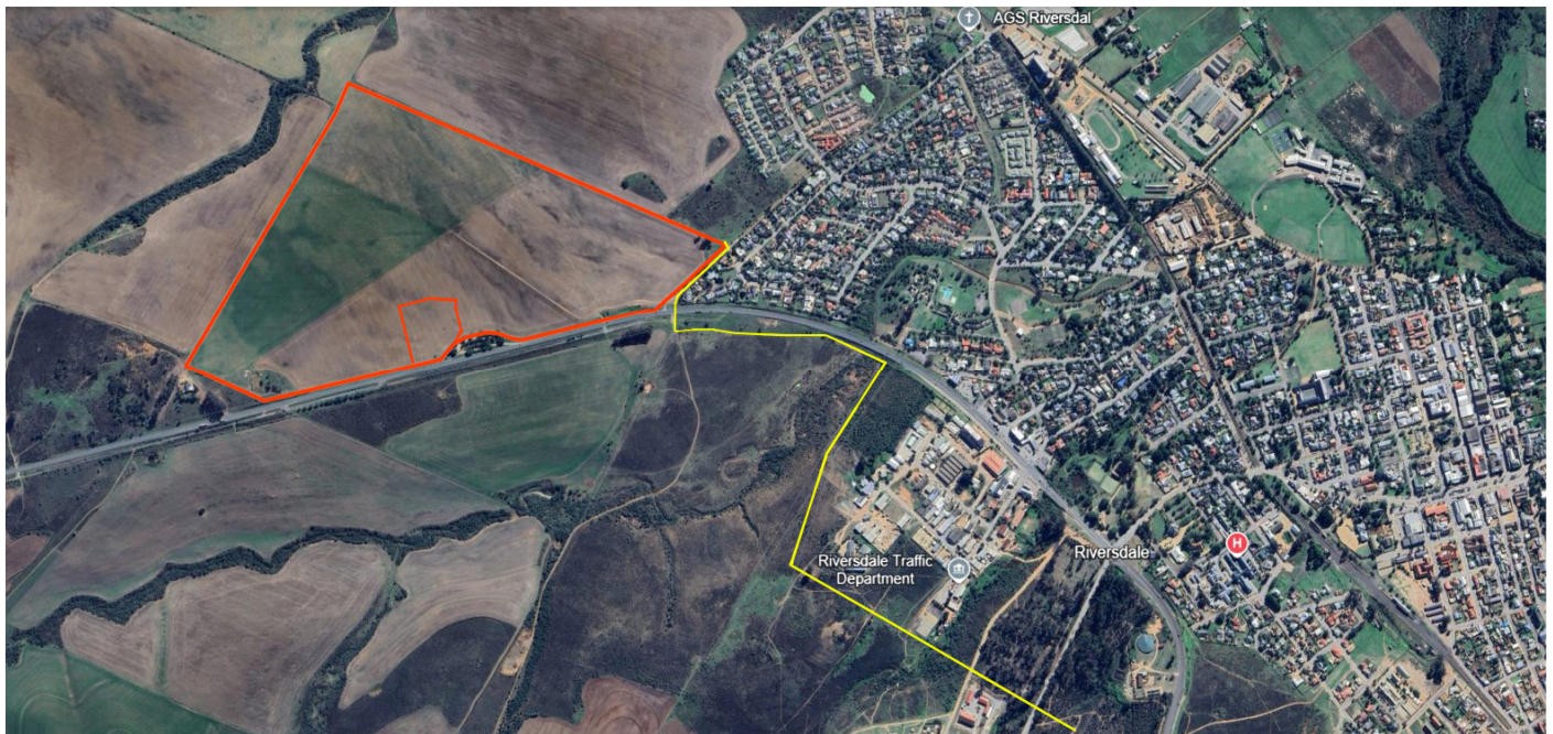
Figure 1: Approximate location of electrical service infrastructure to site (not to scale) shown by yellow lines.
