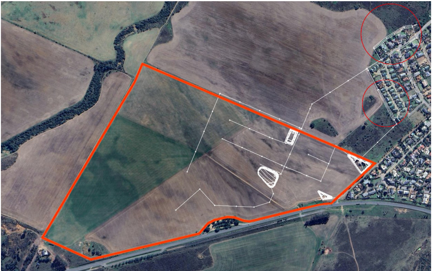
Figure 4: Position of proposed storm water infrastructure and detention structures.
