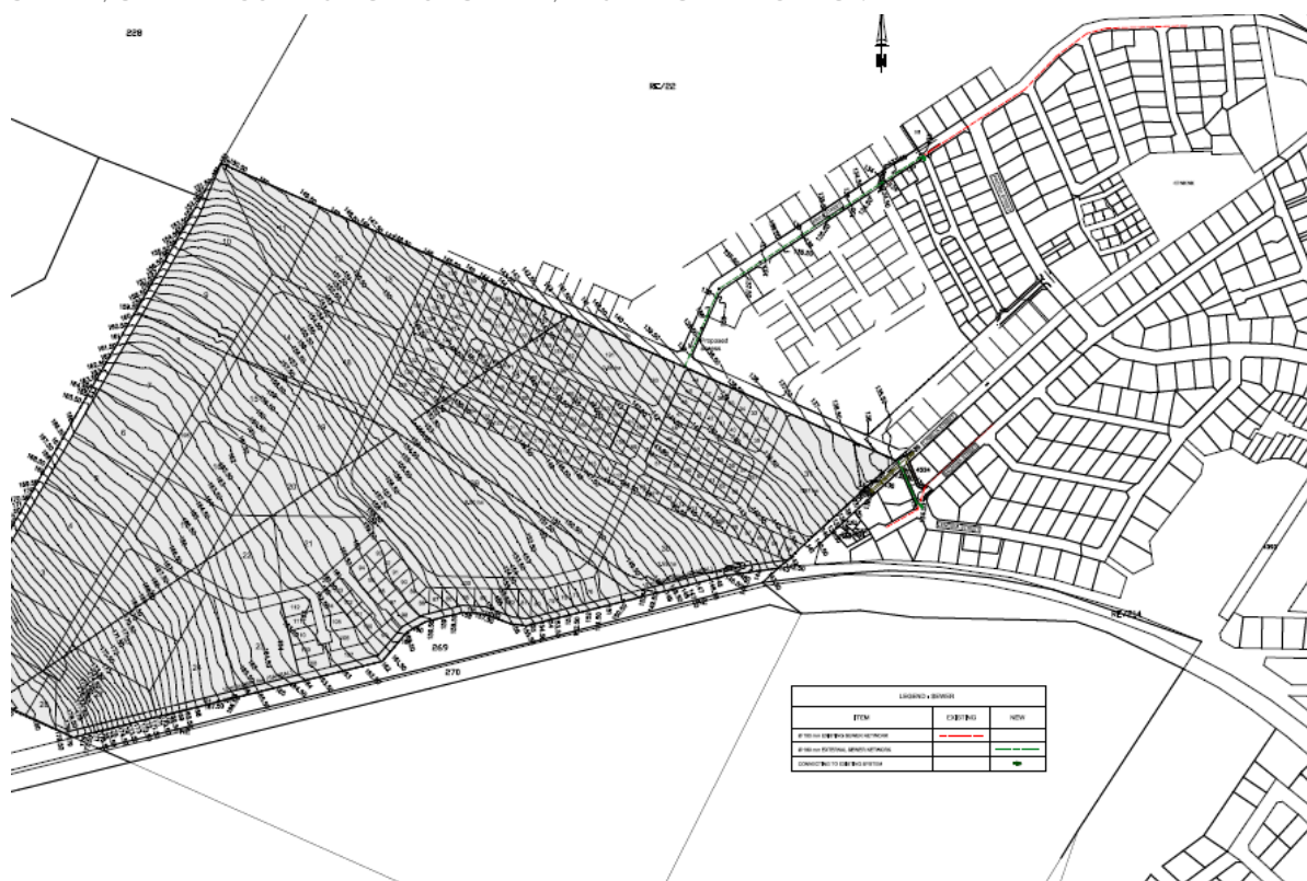
Figure 5. Proposed External Sewer Infrastructure (indicated in green)
