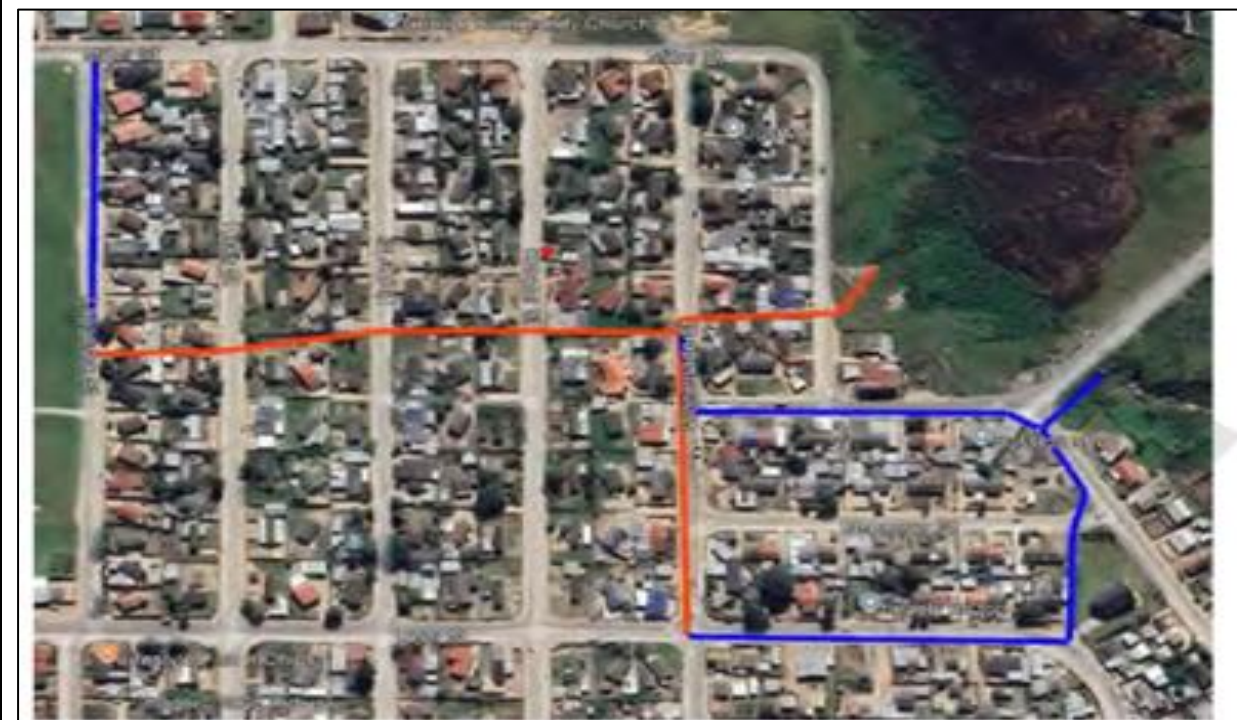
Figure 7: Possible rerouting of Woltemade Outlet Pipe.
