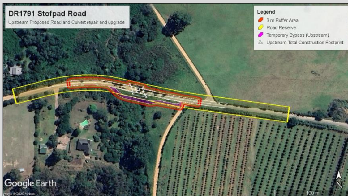
Figure 30. Proposed by-pass infrastructure (upstream)
