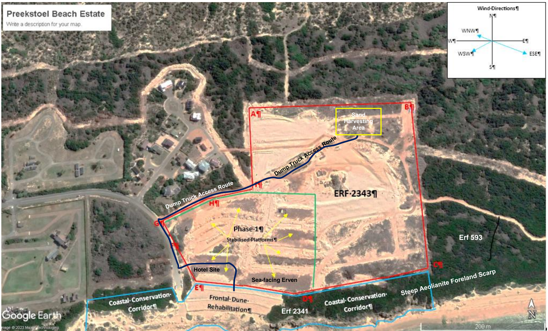
FIGURE 1: Preekstoel Beach Estate, showing the stabilised building platforms, the transformed Frontal Dune System, the Sand Harvesting Area, the Dump Truck Access Route to the frontal dune and the Coastal Conservation Corridor (Erf 2341).
