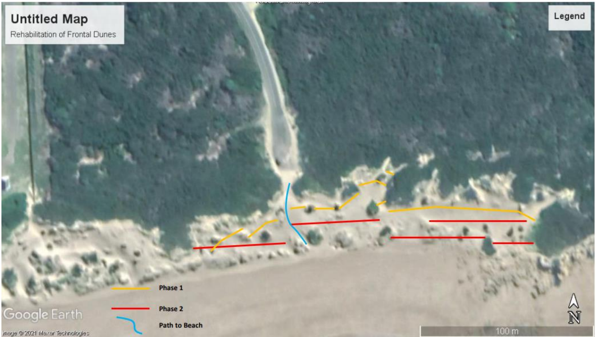
FIGURE 5: Phased Approach for the Rehabilitation of the Preekstoel Frontal Dune System (Google Image dated 10 April 2019) (Note: this methodology was abandoned because of the low accumulation of sand by the erected brushwood fences).
