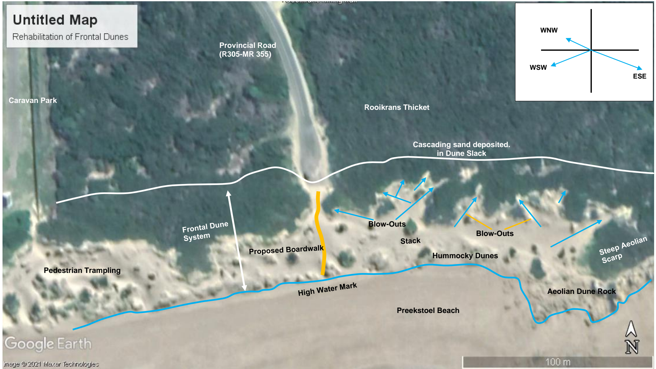
FIGURE 4: Google Image of the Badly Eroded Preekstoel Beach Estate Frontal Dune System (10 April 2019)
