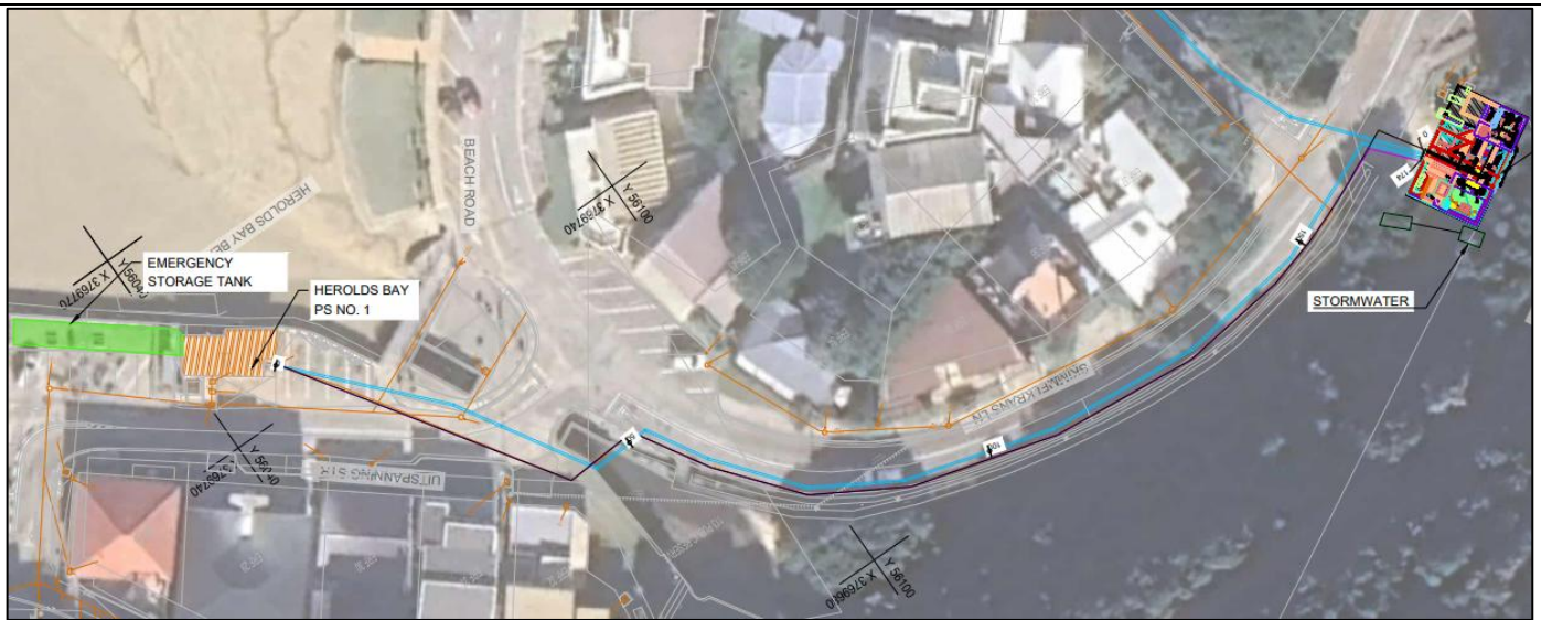
Figure 2: Existing (black) and proposed (blue) pipeline between PS1 and PS4
