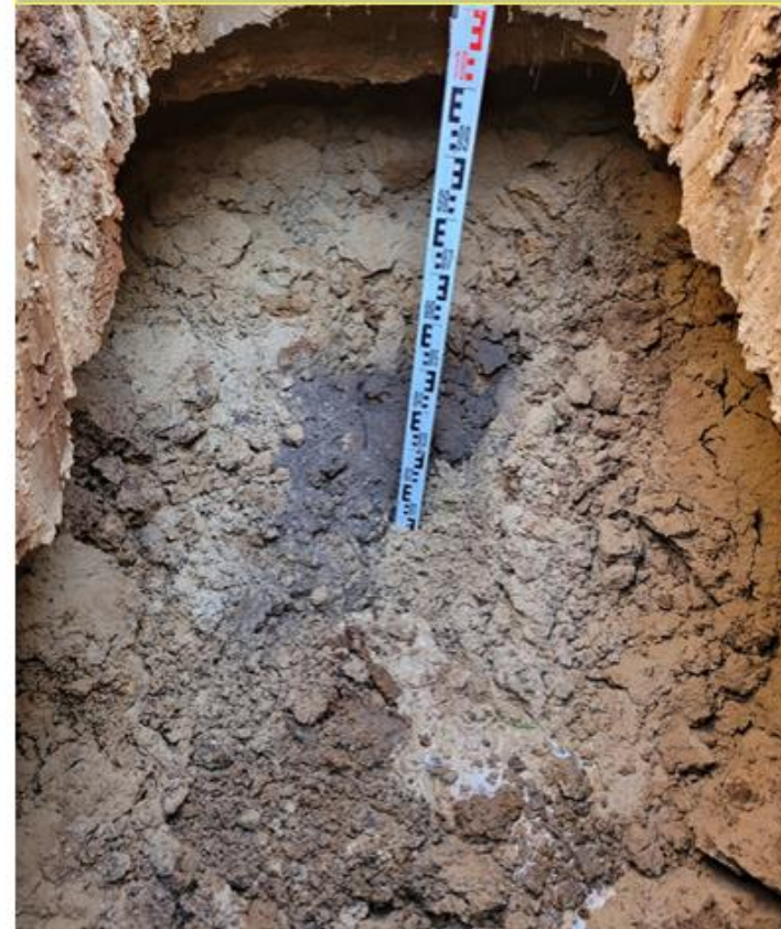
Base of TP13 depicting water seepage and subsequent sidewall instability
