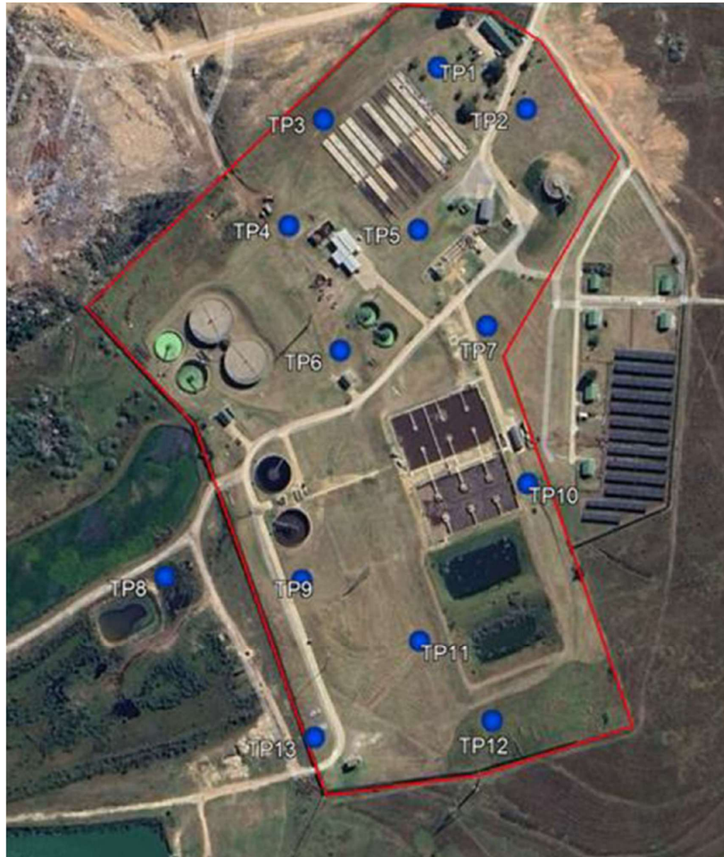
Figure 3: Trial Pit Locations
