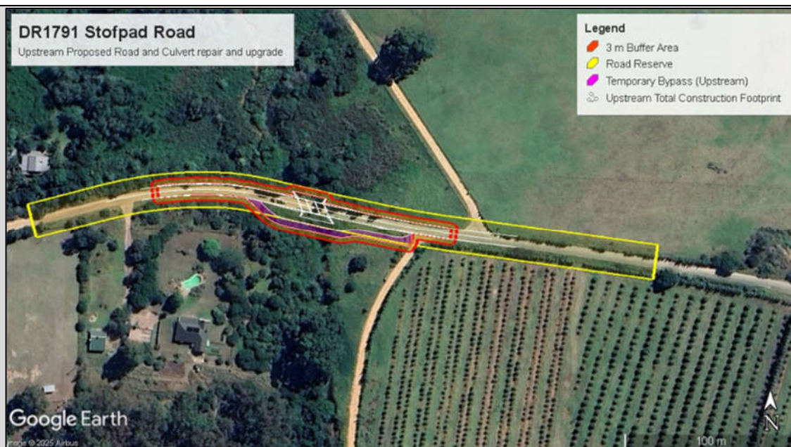
Figure 30. Proposed by-pass infrastructure (upstream)
