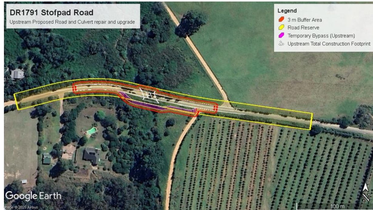
Figure 4. Proposed construction works of the temporary deviation road along DR1791, Wittedrift) (upstream).
