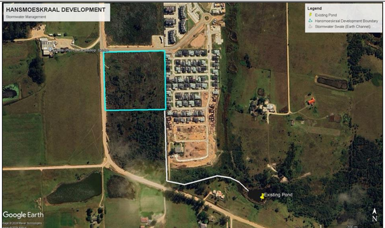
Figure 3: Proposed Stormwater Management Swale
