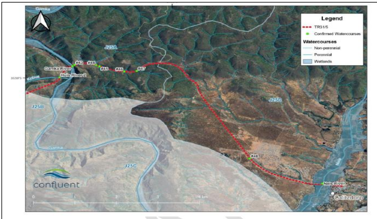
Figure 6: Confirmed watercourses in quaternaries J25A and J25D where maintenance of culverts or bridges could be required.
