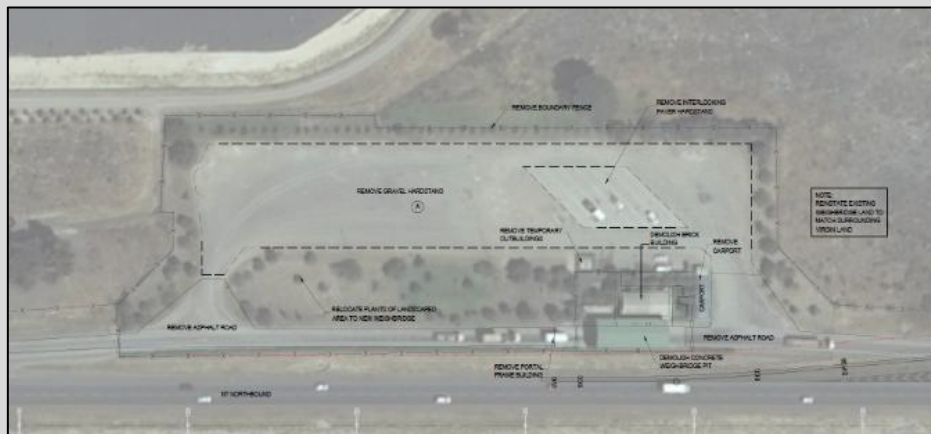
Figure 6. The Demolition plan for the existing weighbridge facility after the new weighbridge is established.
