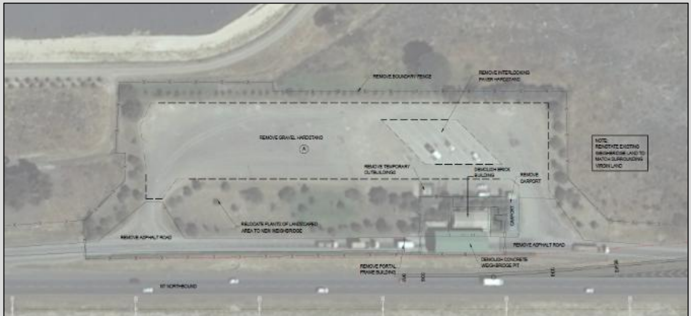
Figure 5. The Demolition plan for the existing weighbridge facility after the new weighbridge is established.
